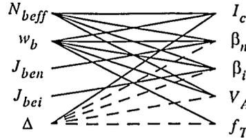
Figure 5: Dependencies between  $p$  and  $e$  for BJTs (dashed lines are weak dependence).
