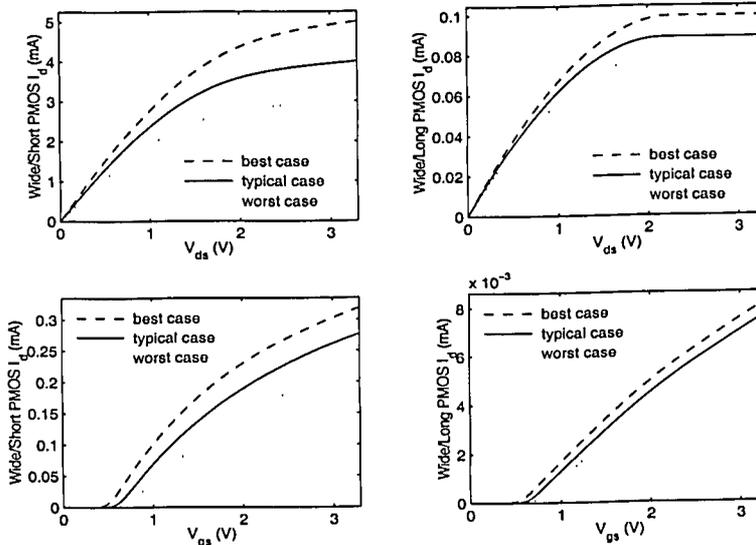
Figure 3:  $I_d(V_d)$  and  $I_d(V_g)$  variation in generic case statistical models.
