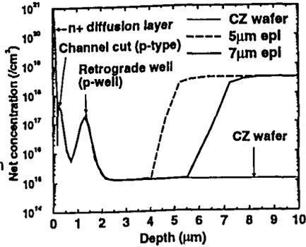
Figure 2: Simulated dopant profile to ward depth direction.
