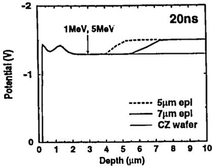
Figure 9: Potential profile in the memory cell at 20ns after a quarter alpha-particle strike.
