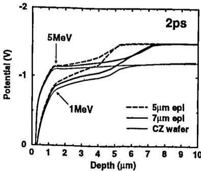
Figure 7: Potential profile in the memory cell at 2ps after a quarter alpha-particle strike.
