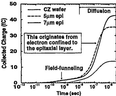
Figure 3: Transient charge-collection behavior in the TEG due to a quarter alpha-particle strike with 5 MeV energy.
