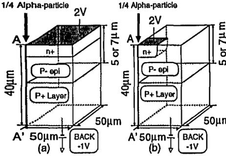
Figure 1: Schematic of the simulated structures, (a) TEG (Test Element Group) and (b) a memory cell.
