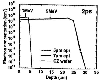
Figure 8: Electron distribution in the memory cell at 2ps after a quarter alpha-particle strike.
