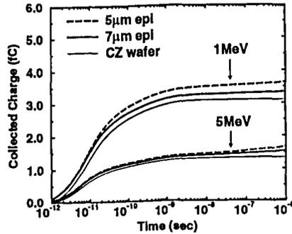
Figure 4: Transient charge-collection behavior in the memory cell due to a quarter alpha-particle strike with 1MeV or 5 MeV energy.
