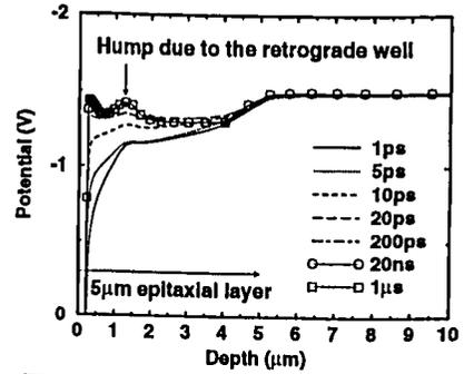
Figure 6: Transient potential distribution in the memory cell after a quarter alpha-particle strike with 5 MeV.
