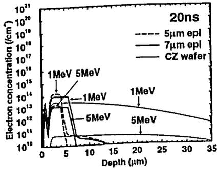
Figure 10: Electron distribution in the memory cell at 20ns after a quarter alpha-particle strike.
