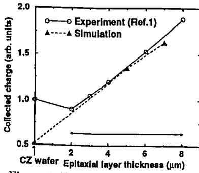
Figure 5: Epitaxial layer thickness dependence of charge-collection in the TEG.
