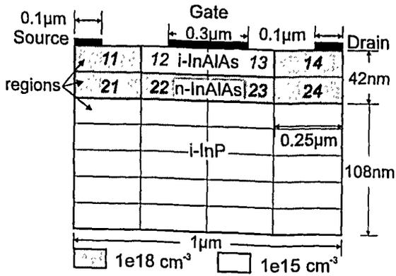
Figure 4: The investigated device structure and geometrical discretization of the spatially resolved distribution functions.
