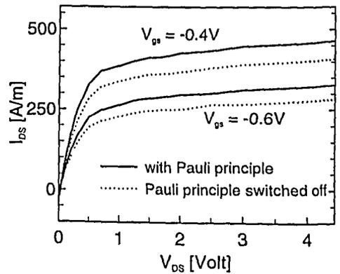
Figure 7: Calculated I-V characteristics of the investigated HEMT.
