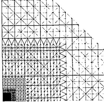
Figure 1: BZ cut ( $k_z = 0$ ,  $0 \leq k_x, k_y \leq 2\pi / a_{Si}$ ) of the tetrahedral mesh used in the case of variable discretization for the first valence band.  $N_{DIV}$  varies from 16 to 256.
