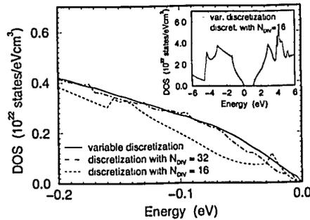
Figure 2: Density of states near the band edge of the valence band for different mesh refinements. Inset: DOS on a larger scale.
