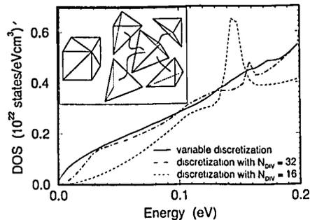
Figure 3: Density of states near the band edge of the conduction band for different mesh refinements. Note that the conduction band minimum has been shifted to the origin by the bandgap energy. Inset: Set of 5 tetrahedra building a regular cube.
