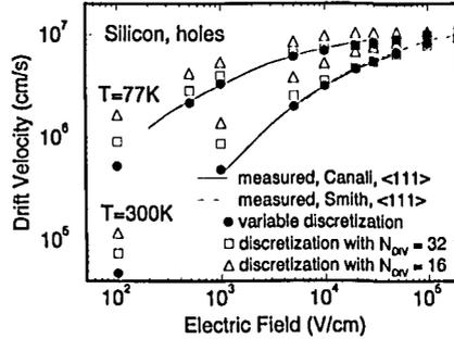
Figure 4: Hole drift velocity versus field. The experimental data is from [14] (solid line), and [15] (dot-dashed line). FBMC transport parameters:  $D_{AC} = 3.65$  eV,  $v_s = 6540$  m/s,  $D_{OP} = 9.5 \cdot 10^{10}$  eV/m,  $\hbar\omega_{OP} = 63$  meV. The FBMC statistical error is  $< 5\%$  except for the values at  $10^2$  V/cm given in Table 2. The confidence level is 99.7%.
