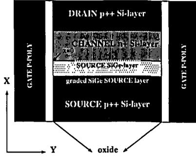
Figure 1: Schematic view of the Si/SiGe vertical pMOSFET
