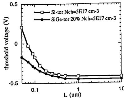
Figure 4:  $V_T$  as a function of the channel length
