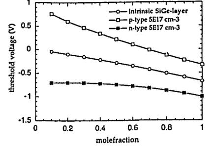
Figure 2:  $V_T$  as a function of the molefraction for different doping concentrations of the SiGe-layer
