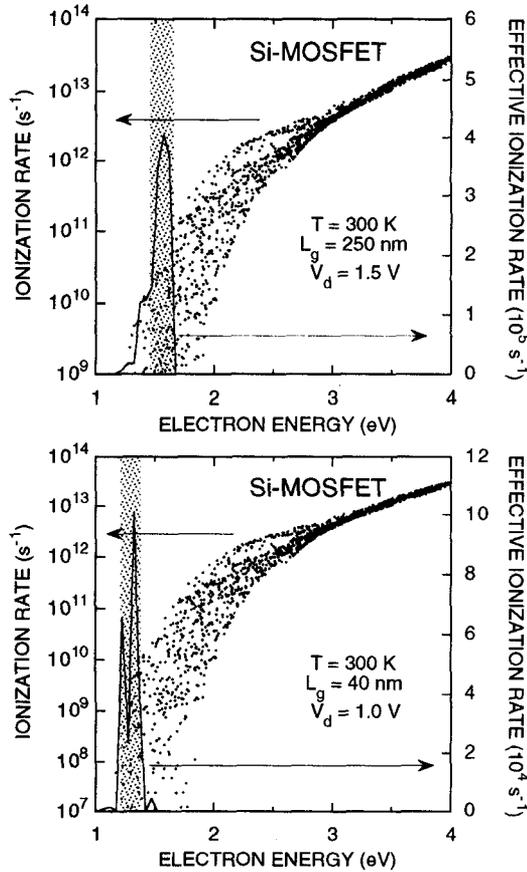
Fig. 2. Effective ionization rates in Si-MOSFET's with  $L_g = 250$  and  $40$  nm (solid curves). The shaded regions schematically represent the width of the effective ionization rates. The wave-vector-dependent ionization rates are also plotted with dots as a function electron wave-vector.
