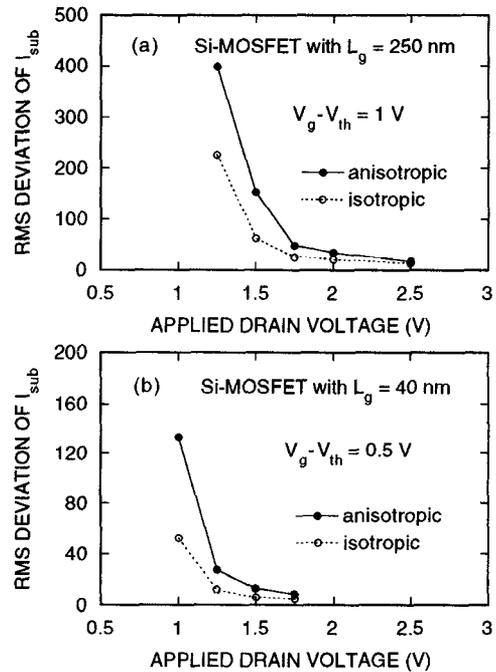
Fig. 3. Normalized standard deviation (root-mean-square deviation) of the substrate currents in Si-MOSFET's as a function of the applied drain voltage. The solid and dotted lines represent the results when the anisotropic and isotropic ionization rates, respectively, are used in the simulations.
