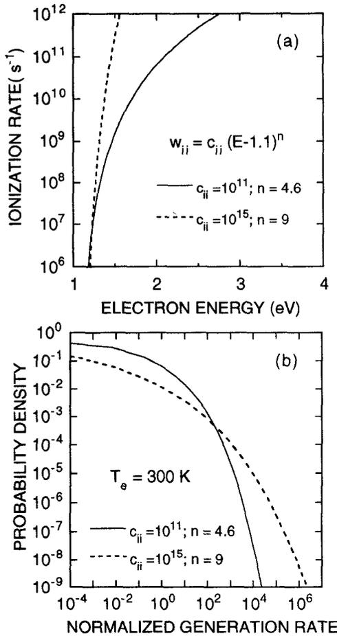
Fig. 1. (a) Impact ionization rates evaluated from the Keldysh formula with two different parameters: soft ionization threshold (solid curve) and hard ionization threshold (dashed curve). (b) Probability density of hole generation rate. The hole generation rate is normalized by the averaged generation rate corresponding to the two different ionization rates given in (a).
