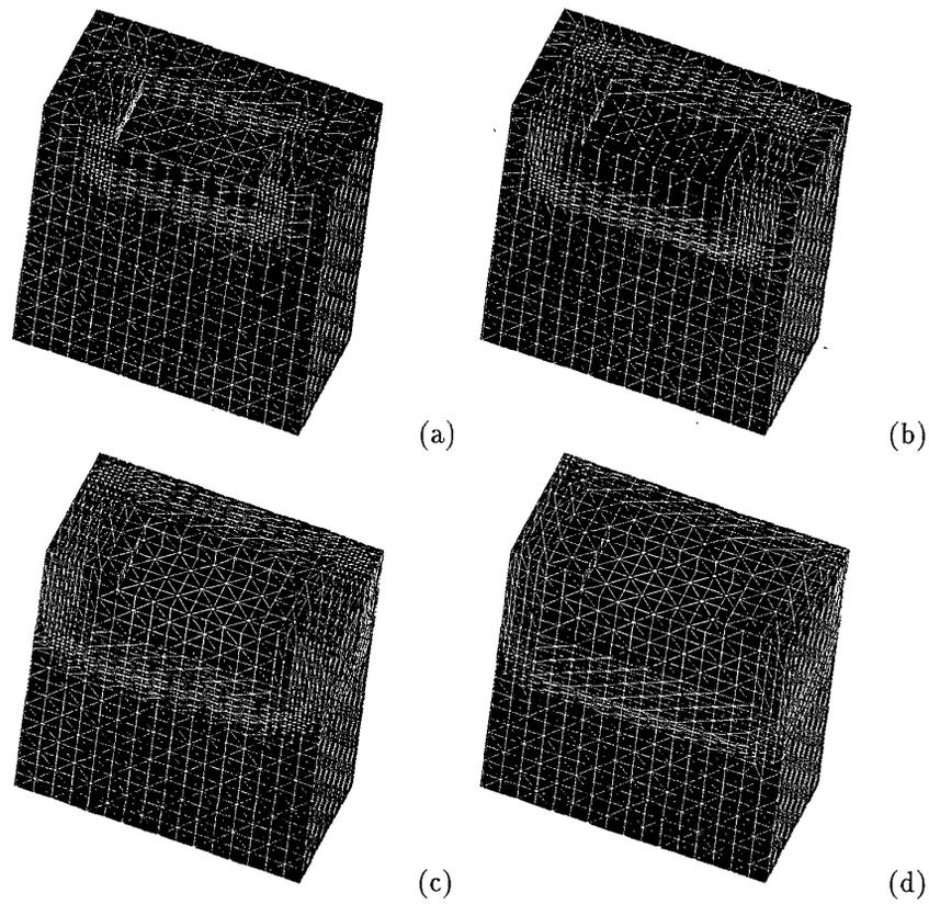
Figure 1: Boron diffusion in a hole structure at 1100 °C. The four meshes are a) initial mesh ( $t = 0$  seconds), b) adapted mesh at  $t = 240$  sec, c) adapted mesh at  $t = 480$  sec, d) adapted mesh at  $t = 720$  sec, respectively.
