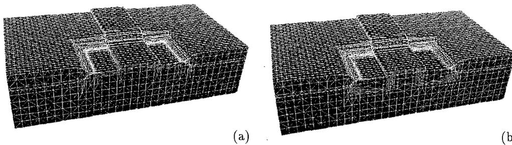
Figure 2: Boron diffusion in a MOSFET at 1100 °C. a) initial mesh. b) final mesh at  $t = 900$  sec.
