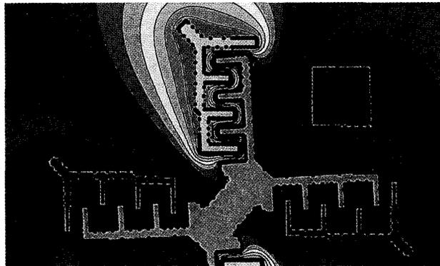
Fig. 2. Potential distribution and automatically adapted mesh. The marked positions at the interfaces indicate boundary nodes.
