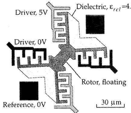
Fig. 1. Layout and boundary conditions of an electrostatically actuated MEMS gyroscope.
