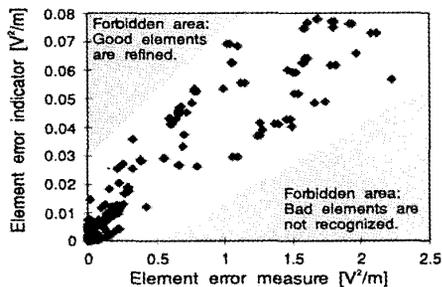
Fig. 3. Indicator value versus error measure for each element (constant elements, 3 μm length).
