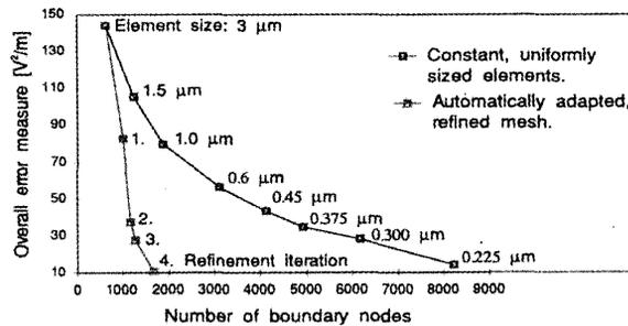
Fig. 4. Overall error measure vs. simulation size for different mesh refinement strategies.
