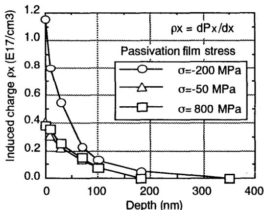
Fig. 3 Piezoelectric charge distribution at gate edge
