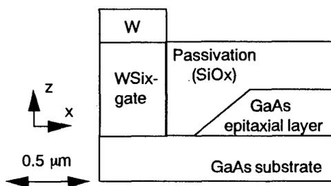
Fig. 1 Model structure of GaAs FET
