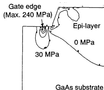
Fig. 2 Predicted stress distribution in GaAs substrate
