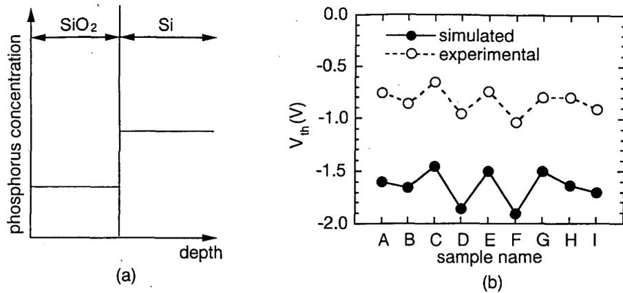
Fig. 1. (a) Schematic diagram of final phosphorus distribution based on ordinary model. (b) Simulated results for threshold voltage of p-channel MOSFETs.
