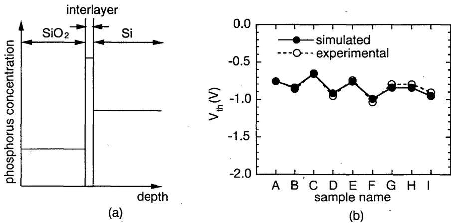
Fig. 2. (a) Schematic diagram of proposed phosphorus pile-up model. (b) Simulated results for threshold voltage of p-channel MOSFETs.
