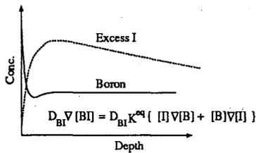
Figure 3: Figure for describing B pileup due to excess interstitial-Si concentration gradient  $\nabla[I]$ .
