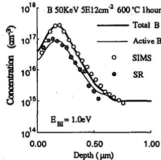
Figure 7: Experimental and calculation results for the low dose boron implantation and low temperature anneal experiment. The best fit was obtained using  $E_{BI}=1.0\text{eV}$ .  $D_I$  was reduced to 1/100 considering I-clustering effectively.
