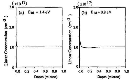
Figure 2: One-dimensional test calculation results for the boron surface pileup due to excess interstitial silicon (I) with different  $E_{BI}$  values. Boron profile: initially flat. Si implantation:  $2.7 \times 10^{13}\text{cm}^{-2}$ , 180keV. Anneal: 800°C, 1hour.  $D_I/K_I=0.01\mu\text{m}$ . Smaller  $E_{BI}$  gives larger pileup amount.
