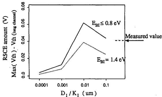
Figure 6: Dependence of surface recombination rate ( $K_I$ ) and  $E_{BI}$  on the calculated RSCE amount.
