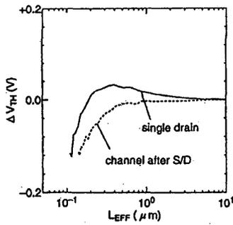
Figure 1: Experimental data for the nMOSFET reverse short channel effect (RSCE) [3], where channel B profile: initially flat from surface to  $0.2\mu\text{m}$  deep,  $t_{ox}=5\text{nm}$ , S/D implantation: Arsenic,  $1\sim 5 \times 10^{15}\text{cm}^{-2}$  10keV, anneal: FA(800°C) or RTA(1000°C). Dashed line shows the data for which the channel B was implanted after S/D annealing [3], supporting that S/D implantation causes this RSCE.
