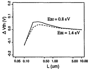
Figure 4: Two-dimensional calculation results for the reverse short channel effect with different  $E_{BI}$  values.  $D_I/K_I$  was set to  $0.01\mu\text{m}$ .
