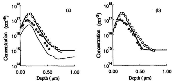
Figure 8: Comparison between calculation results and experimental data for the low dose boron low temperature annealing conditions. (a)  $E_{BI}=1.4\text{eV}$ , too-low activation. (b)  $E_{BI}=0.8\text{eV}$ , all the boron erroneously became active. Lines and symbols are the same as those in Fig.7
