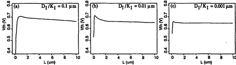
Figure 5: Calculation results for the  $V_{th}$  (threshold voltage)- $L$  (channel length) characteristics with different surface recombination rate ( $K_I$ ) values for the interstitial silicon. Annealing for 1hour at 800°C.
