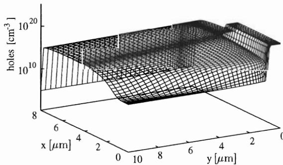
Figure 5: Hole distribution at high forward bias
