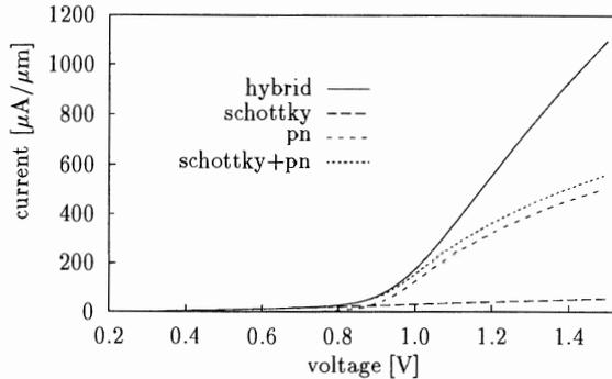
Figure 4: Forward I/V characteristics
