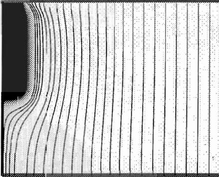
Figure 2: Current pattern at low forward bias
