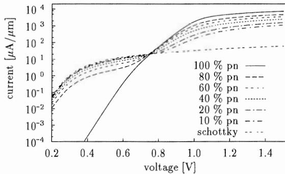
Figure 6: I/V characteristics at various pn/Schottky ratios
