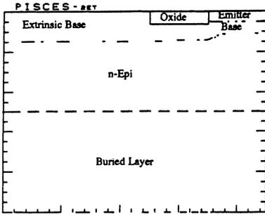
Figure 1. Cross-section of a silicon bipolar transistor used for harmonic balance PISCES analysis.
