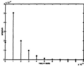
Figure 2. Collector current spectrum under a large-signal single-tone sinusoidal input.
