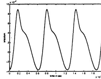
Figure 3. Time-domain representation of Figure 2. The harmonic balance run is drawn as a solid line, whereas a PISCES transient run is drawn dashed. No difference between the two can be seen.
