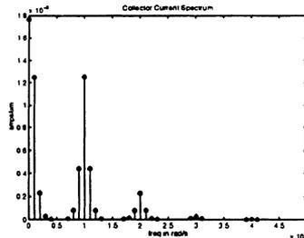
Figure 4. Collector current spectrum under a two-tone intermodulation distortion test.
