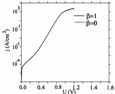
Fig. 1 : Calculated IU characteristics for a  $n^+p$ -diode and two values of  $\beta$ .
