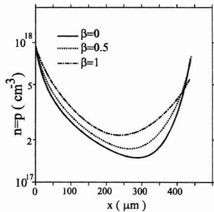
Fig. 3: Charge carrier distribution in the base of the diode from Fig. 2 at  $j=1000 \text{ A}/\text{cm}^2$
