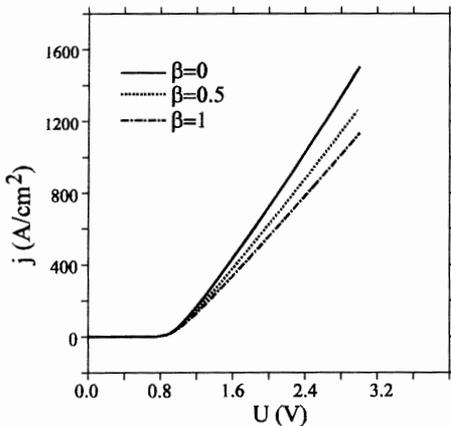
Fig. 2: Calculated current-voltage characteristics of a long base *psn*-diode
