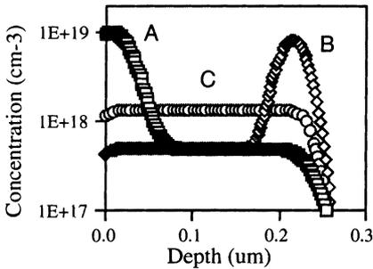
Figure 2: Three extreme cases of LDD profiles with identical sheet resistance and identical junction depth used for MINIMOS simulations of the I-V characteristics in the triode regime.
