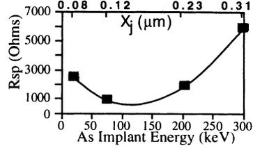
Figure 5: Spreading resistance  $R_{sp}$  for As LDD implants as a function of implant energy. (LDD dose adjusted to keep  $R_{sh}$  constant.) Reversal effect near  $\chi_j = 0.15\mu\text{m}$ , not predicted by previous models, is clearly seen.
