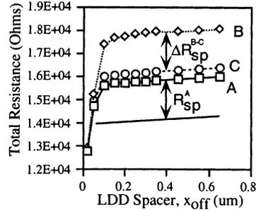
Figure 3: MINIMOS simulations of total MOSFET resistance ( $V_D = 0.1\text{V}$ ,  $V + G = V_T + 0.2\text{V}$ ,  $L = 0.5\mu\text{m}$ ,  $W = 1.0\mu\text{m}$ ) versus spacer length,  $x_{off}$ , for LDD profiles from Fig.2. Beginning at  $x_{off} = 0.04\mu\text{m}$  LDD regions are completely buried under the  $n^+$  S/D regions.
