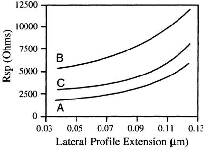
Figure 4: Spreading resistance  $R_{sp}$  for profiles A, B, C (Fig.2) as a function of lateral profile extension (slope). In agreement with ref.[1] steep lateral junctions minimize the spreading resistance. However, vertical profile variations are more significant than realistic lateral profile variations.
