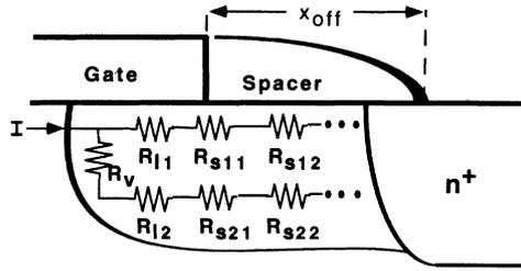
Figure 1: A resistor network describing the spreading resistance in the LDD region. Resistors  $R_v$ ,  $R_{l1}$ , and  $R_{s11}$  depend upon gate bias.
