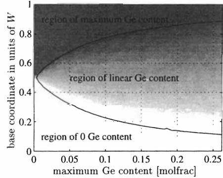
Fig. 2: Location of the three different parts of optimum Ge profiles and the points where they meet with their dependence on maximum Ge content.
