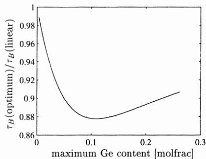
Fig. 4: Ratio of  $\tau_B$  for optimum and linear profile for maximum Ge contents from 0 to 25%.
