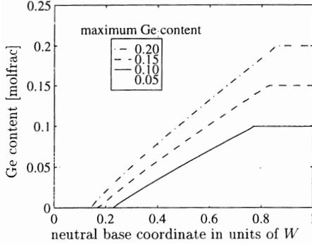
Fig. 1: Four examples of optimum Ge profiles for different values of maximum Ge content which are given in the legend.
