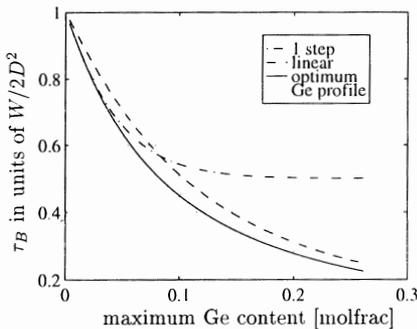
Fig. 3: Dependence of neutral base transit time  $\tau_B$  on maximum Ge content for different Ge profile types.
