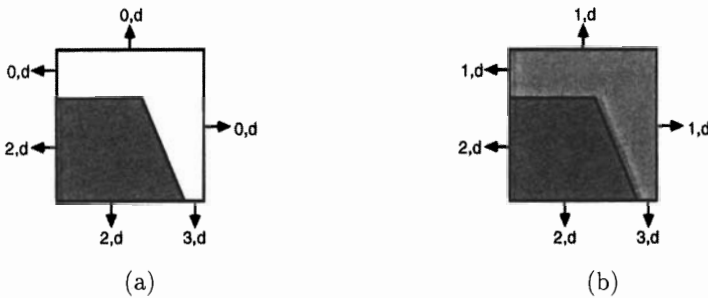
Figure 2: Extraction and modification of the polygonal geometry for the redeposition simulation of the cell in the center of figure 1b and 1c. The vectors at the borders give the material types outside of the cell and the classifications of the neighboring cells. (d...deposited)
