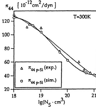
Fig. 1: Comparison of measured [3] and calculated piezoresistive shear coefficient  $\Pi_{44}$  in p-doped silicon versus concentration  $N_s$  of the diffused piezoresistive layer.
