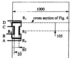
Fig. 3: Top view of a microresonator structure with piezoresistive readout (lengths in  $\mu\text{m}$ ).
