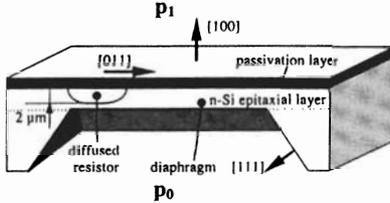
Fig. 4: Cross section of the simulated pressure sensor, showing crystal orientations and the location of the piezoresistors.  $p_0$  is the reference pressure,  $p_1$  the measurand.
