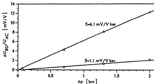
Fig. 7: Sensor response of the analyzed diaphragm structures (Δ structure from Fig. 2, o structure from Fig. 3).
