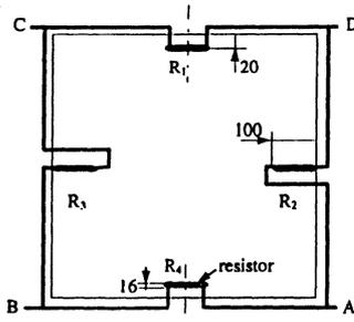
Fig. 2: Top view of a sensor structure for pressure measurement [4] (lengths in  $\mu\text{m}$ ).
