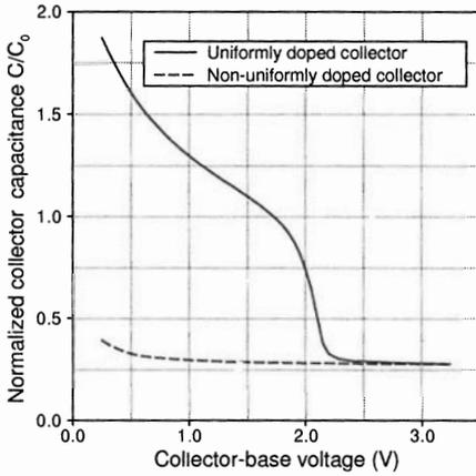
Figure 3: The normalized collector capacitance versus collector-base voltage for HBTs with buried subcollector and different collector doping profiles.
