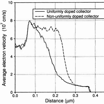
Figure 5: Average electron drift velocity corresponding to HBTs with conventional (solid curve) and proposed (dashed curve) collector structures.
