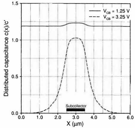
Figure 4: The distributed base-collector capacitance  $c(x)$  as a function of position for HBT with uniformly doped collector structure.
