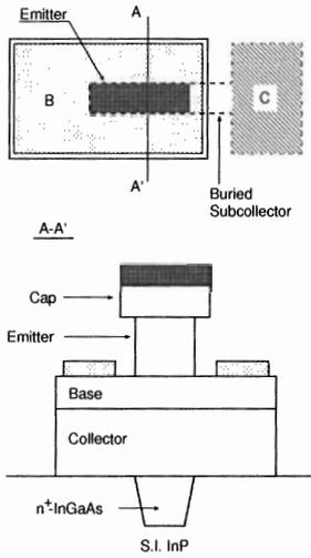
Figure 1: Schematic layout and cross-section of simulated HBT with buried subcollector.
