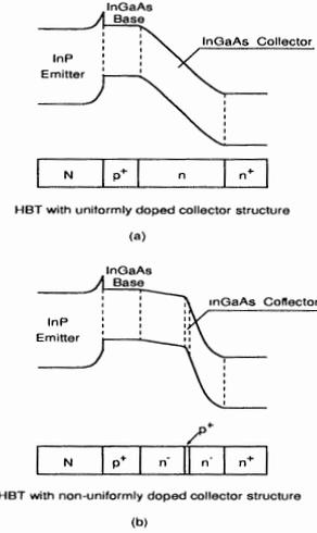
Figure 2: Schematic band diagrams and doping of HBTs with buried subcollector: (a) uniformly doped collector and (b) non-uniformly doped collector.
