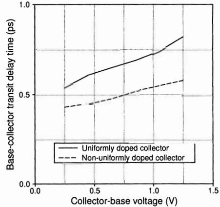
Figure 6: The base-collector transit delay time versus collector-base voltage for HBTs with buried subcollector and different collector doping profiles.
