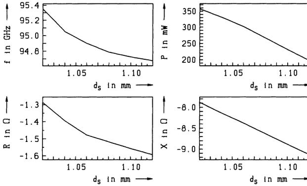
Figure 1: Operating frequency, output power, dynamic resistance and dynamic reactance vs. disc diameter.
