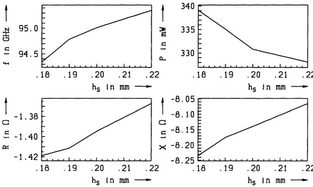
Figure 2: Operating frequency, output power, dynamic resistance and dynamic reactance vs. disc thickness.
