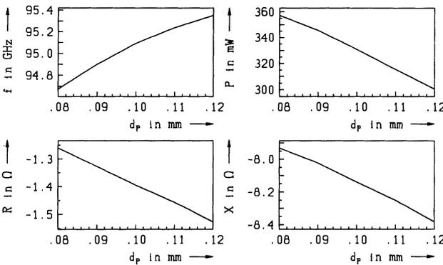
Figure 3: Operating frequency, output power, dynamic resistance and dynamic reactance vs. post diameter.
