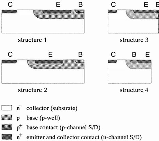
Figure 1: CMOS-compatible BJT structures
