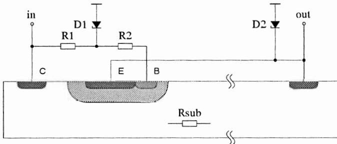
Figure 4: Integration of the protection circuit with structure 3
