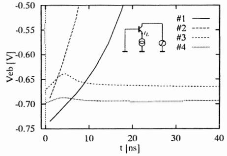
Fig. 8: Voltage overshoot at 80V/us, I=300mA/cm for different structures
