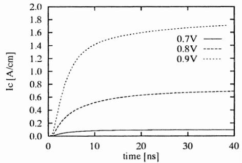
Fig. 10: Turn-on characteristics of structure 4 for different Vbe pulses (tr=1ns, Vce=10)
