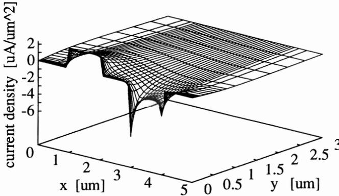
Figure 3:  $y$ -component of electron current density
