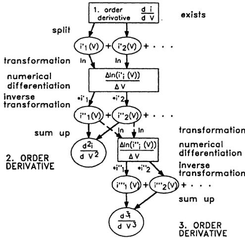
Figure 2: Differentiation scheme for bipolar devices
