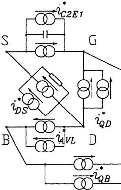
Figure 3: MOST equivalent circuit for distortion analysis
