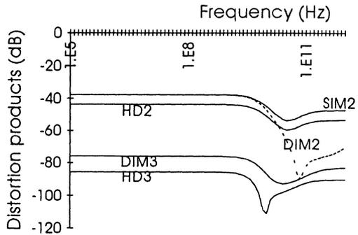
Figure 4: Distortion analysis of a MOST circuit
