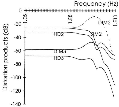
Figure 6: Distortion analysis of a MEXTRAM circuit
