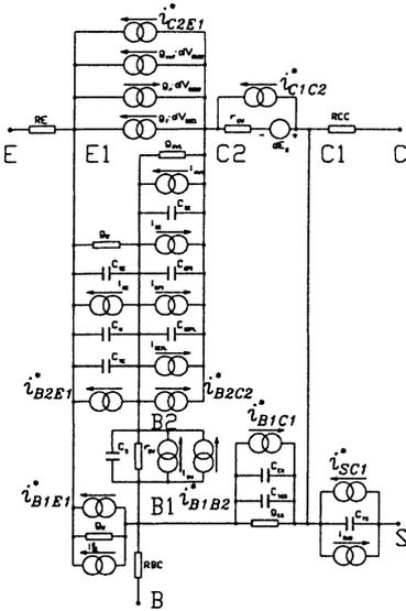
Figure 5: MEXTRAM equivalent circuit for distortion analysis
