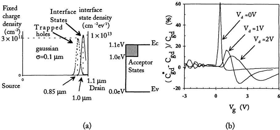
Fig. 5 (a) Assumed spatial distribution and the distribution in the energy band gap of the interface states for the simulated device. (b) Percentage change in simulated  $C_{gd}$  due to trapped holes and acceptor states versus  $V_g$ .
