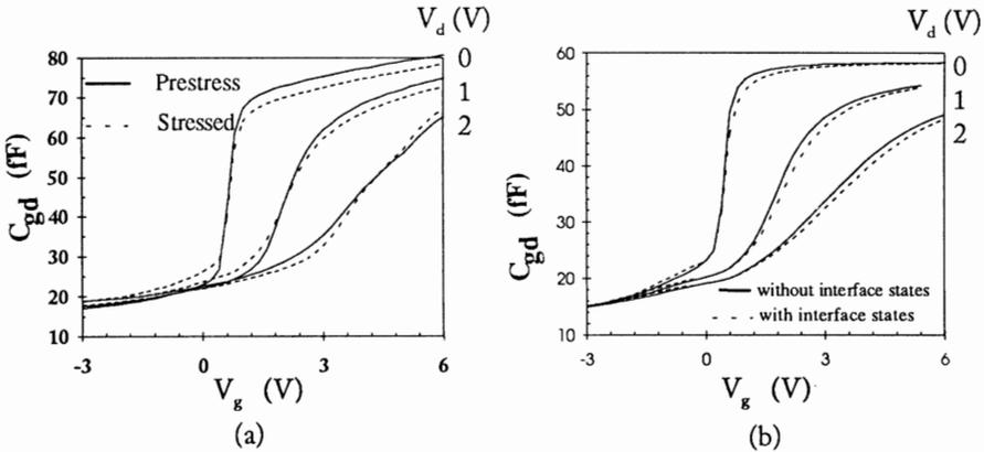
Fig. 1 (a) Measured  $C_{gd}$  versus  $V_g$  for n-MOSFET, stress condition:  $V_d=8$  V,  $V_g=2$  V, stress time=1800s. (b) Simulated  $C_{gd}$  versus  $V_g$  with and without interface states, see Fig. 3 for interface state distribution.
