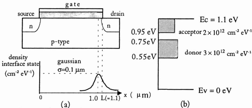
Fig. 3 (a) Assumed spatial distribution and (b) the distribution in the energy band gap of the interface states for the simulated device.
