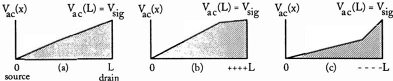
Fig. 2 AC channel potential profile showing the effect of charge in the oxide near drain: (a) with no charge, (b) with positive charge, (c) with negative charge.
