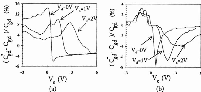
Fig. 4 (a) Percentage change in measured  $C_{gd}$  after stress versus  $V_g$ . (b) Percentage change in simulated  $C_{gd}$  due to interface states versus  $V_g$ .
