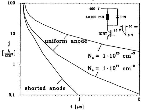
Fig. 7 : Current density during turn-off
