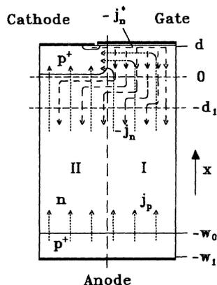
Fig. 1: The two sections of an IGBT
