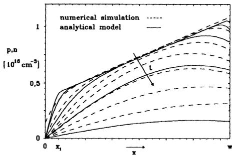
Fig. 5 : Carrier profiles in the neutral base
