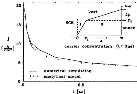
Fig. 4 : Total current density  $j$  during turn-off
