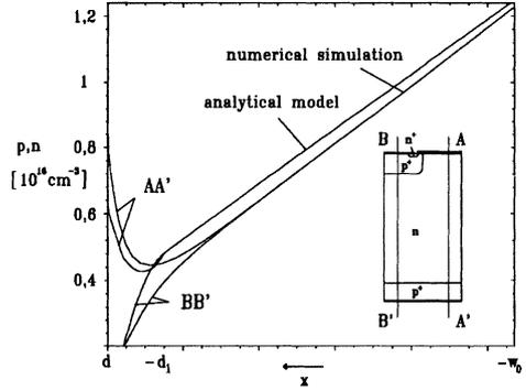
Fig. 2 : Carrier concentration in the IGBT
