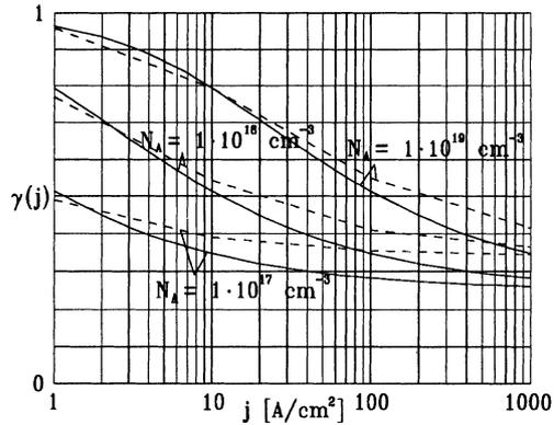
Fig. 3 : Emitter efficiency of uniform p<sup>+</sup>-emitters
