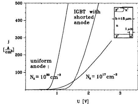
Fig. 6 : IV-characteristic of IGBTs with different anode designs
