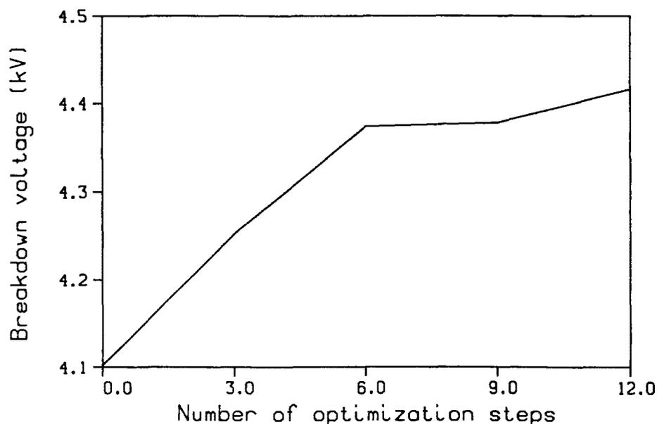
Figure 4: Minimum breakdown voltage within the  $6 \mu\text{m}$  interval of the depth of etching as function of the number of optimization steps
