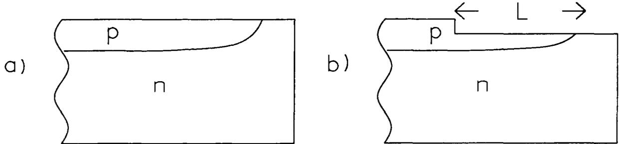
Figure 1: Planar junction termination a) before and b) after etching process
