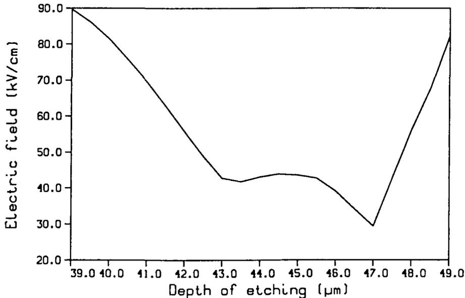
Figure 5: Maximum surface electric field vs. depth of etching after 12 steps of optimization
