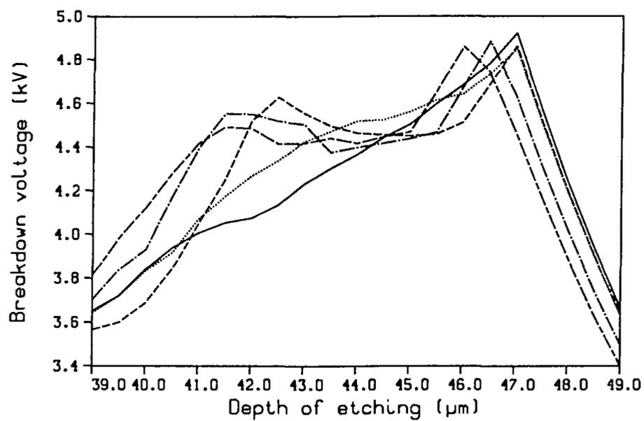
Figure 3: Dependence of the breakdown voltage on the depth of etching at different stages of the optimization
