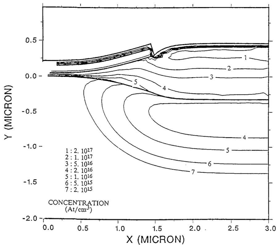
Figure 5: Boron concentration iso-values contours in a LOCOS structure. This simulation includes the stress effects in the oxidation kinetics.
