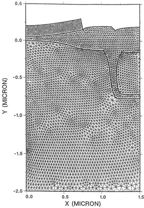
Figure 1: Finite element mesh for the multi-layers process simulation of a trench structure.
