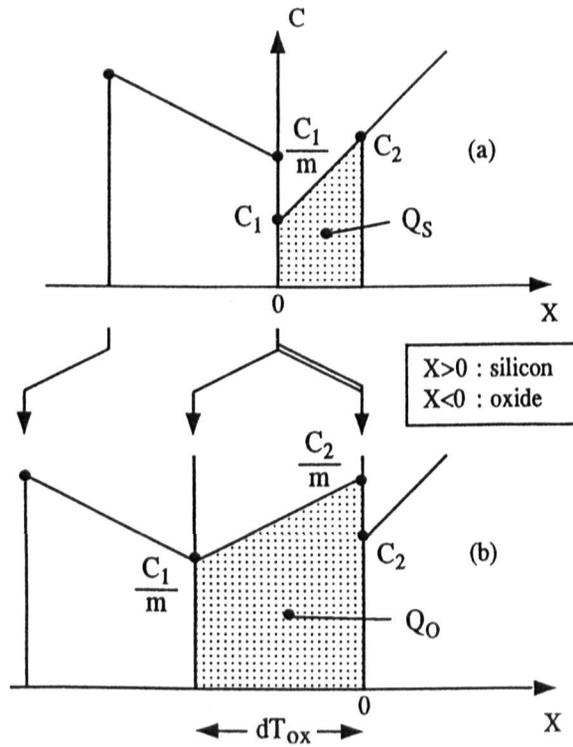
Figure 2: Concentration interpolation scheme for the moving Si/SiO<sub>2</sub> boundary. (a) Before the oxidation step. (b) After the Si/SiO<sub>2</sub> motion corresponding to an oxide growth thickness  $dT_{ox}$ .
