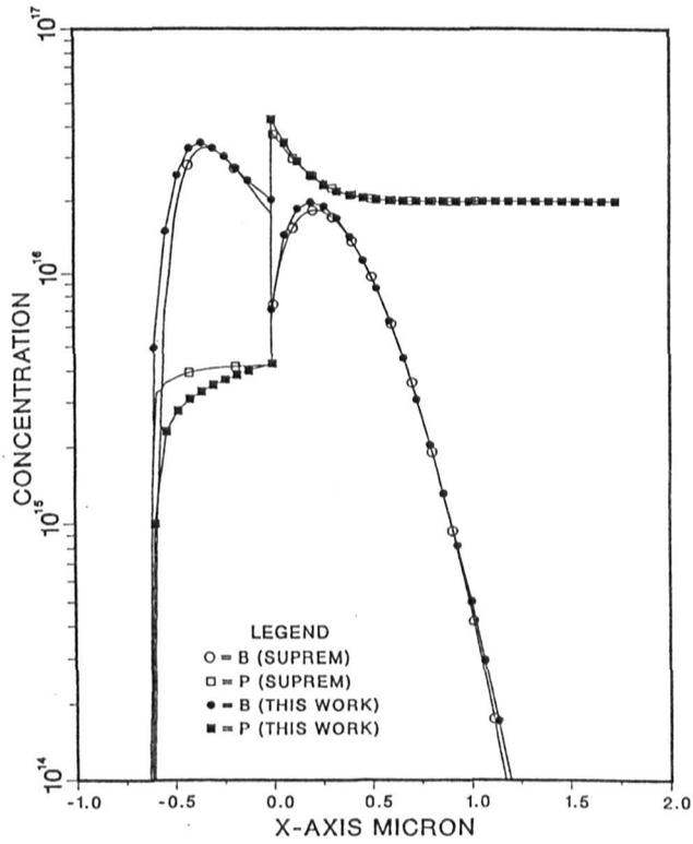
Figure 3: Simulated phosphorus and boron profiles after a wet oxidation, comparison with SUPREM-II results.
