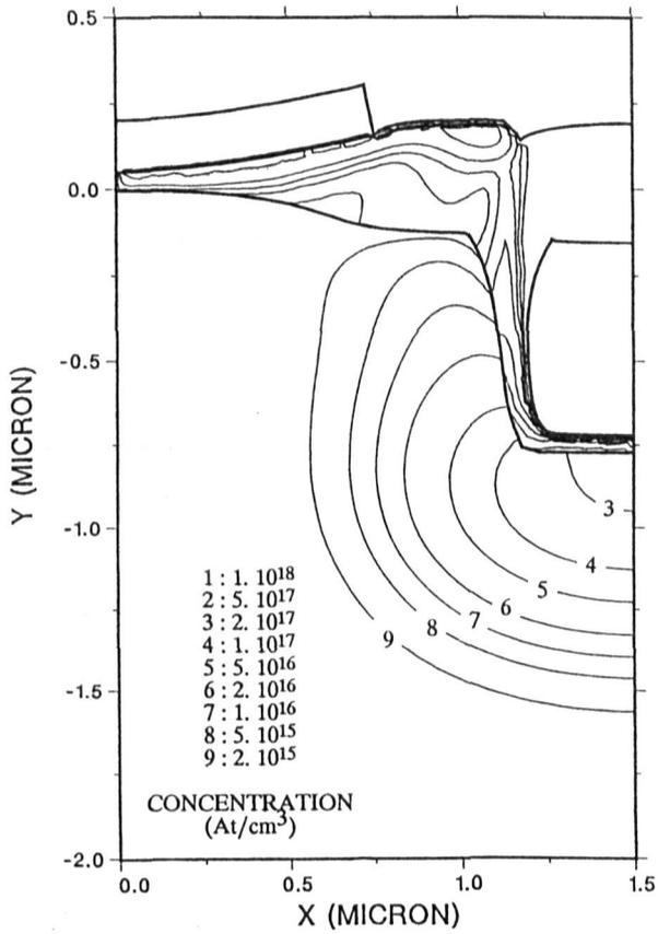
Figure 4: Boron iso-values contours in the structure of fig.1 after the trench oxidation.
