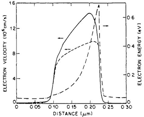
Fig.6 Average electron velocity in the MC (solid) and DD (dashed) case and surface electron energy in the MC solution (dashed-dotted) for  $L_{gate} = 0.15\mu m$ ,  $V_{GS} = 1.5V$ ,  $V_{DS} = 2.0V$ .
