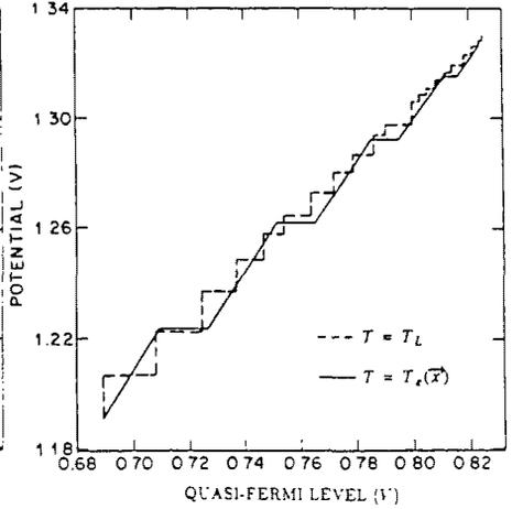
Fig.4 Convergence rates of the point in fig.3 when using the lattice temperature  $T_L$  (dashed line) or the electronic temperature  $T_e$  (solid line) in the non linear Poisson equation.
