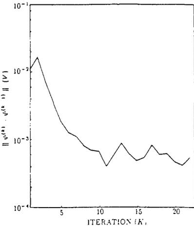
Fig.5 The L-2 norm of the relative error in the electrostatic potential as a function of the number of iterations.
