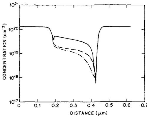
Fig.1 Electron surface concentration for a MOSFET with a gate mask length  $L_{gate} = 0.25 \mu\text{m}$  at  $V_{GS} = 1.5V$ ,  $V_{DS} = 2.0V$  in the DD (solid), non self-consistent MC (dashed-dotted) and self-consistent MC (dashed) case.
