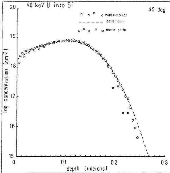
Fig. 3 A comparison of 40keV boron profiles .45 degree incidence.
