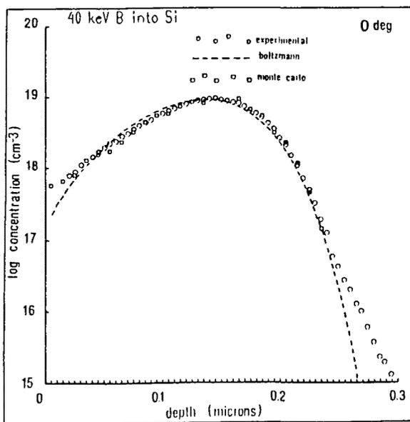
Fig. 2 A comparison of 40keV boron profiles. Normal incidence.
