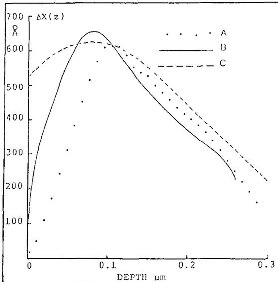
Fig. 6 Depth dependent lateral standard deviation function  $\Delta X(z)$ , (A) experimentally derived, (B) Boltzmann, (C) Monte Carlo. 40keV boron in pre-amorphised silicon.
