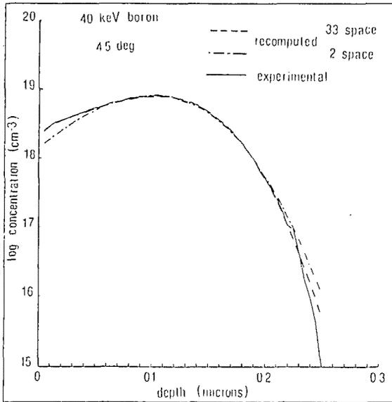
Fig. 5 Recomputed and experimental  $F_{\theta}(z)$ .
