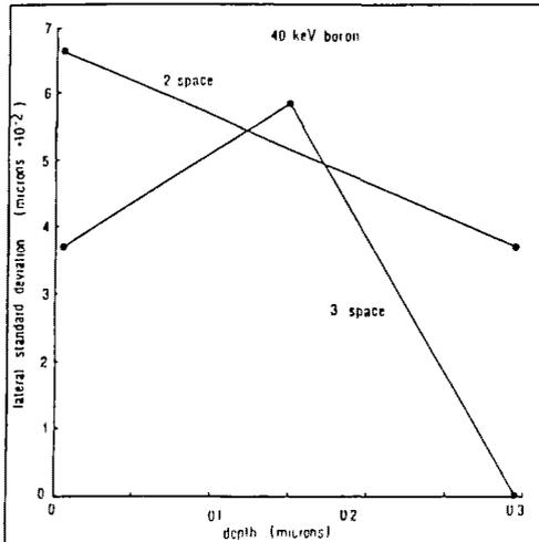
Fig. 4 Linear segment representations of  $\Delta X(z)$  for 40keV boron ions.
