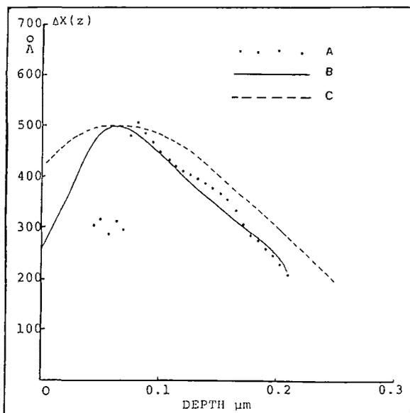
Fig. 7 Depth dependent lateral standard deviation function  $\Delta X(z)$ , (A) experimentally derived, (B) Boltzmann, (C) Monte Carlo. 30keV boron in pre-amorphised silicon.
