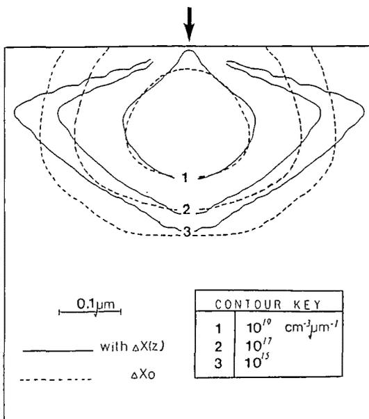
Fig. 8 Reconstruction of two dimensional distribution functions for 40keV boron implanted into amorphous silicon. Dose  $10^{14} \text{ cm}^{-2}$ .
