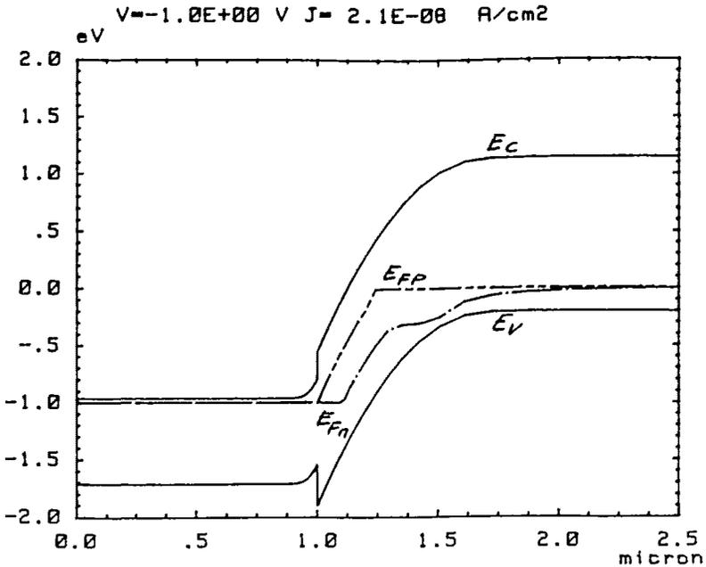
Fig. 3. b) N type InGaAs over P type InP diode under reverse bias
