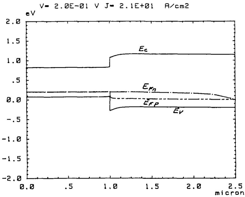
Fig. 2. a) Band diagram of forward bias P - P isotype heterojunction.
