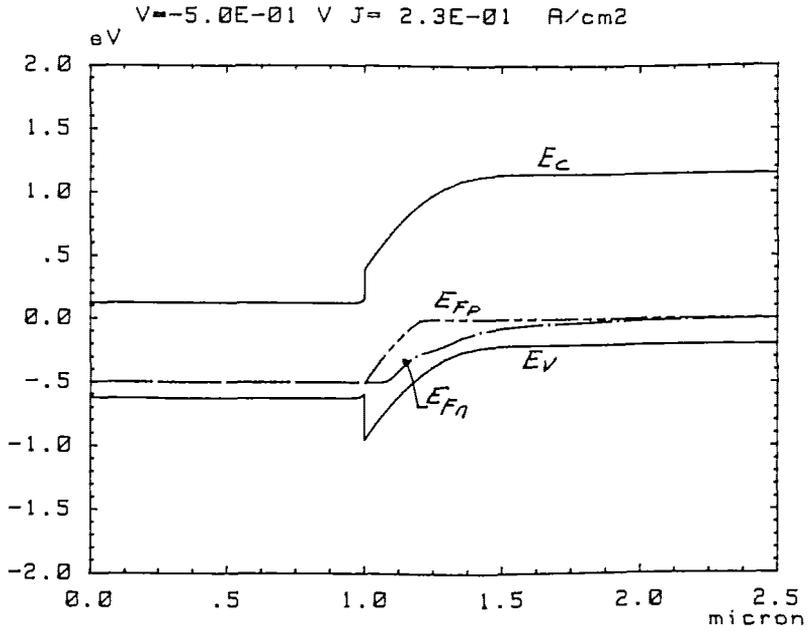
Fig. 2. c) Band diagram of reverse bias P - P isotype heterojunction.
