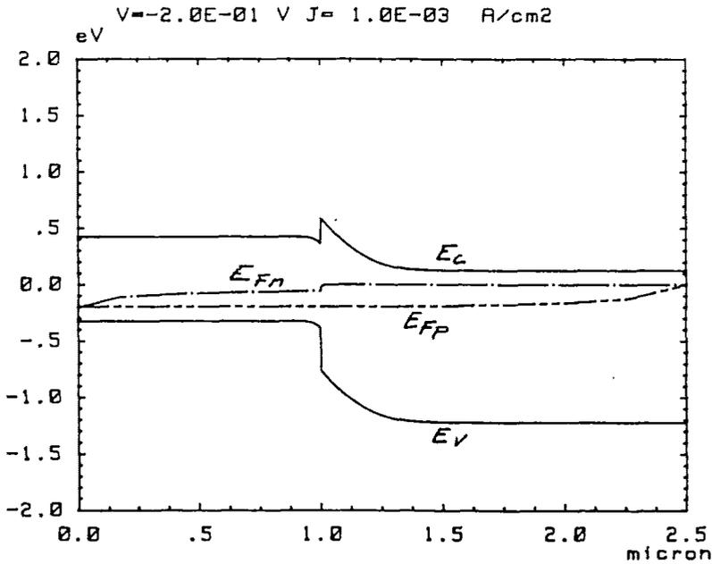
Fig. 4. a) P type InGaAs over N type InP diode under forward bias
