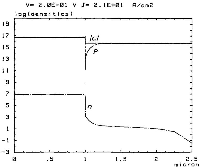
Fig. 2. b) Carrier profiles of forward bias P - P isotype heterojunction.
