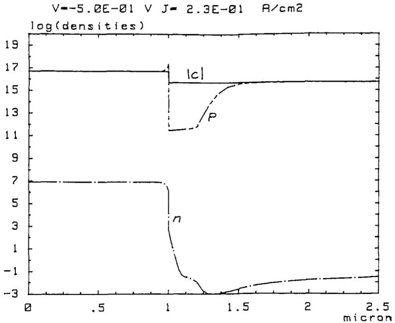
Fig. 2. d) Carrier profiles of reverse bias P - P isotype heterojunction.
