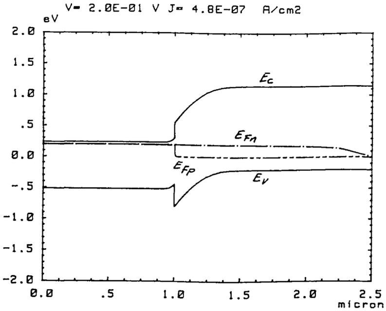
Fig. 3. a) N type InGaAs over P type InP diode under forward bias
