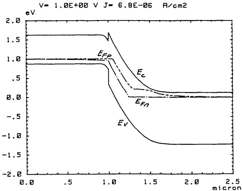
Fig. 4. b) P type InGaAs over N type InP diode under reverse bias
