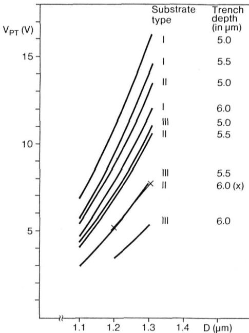
*Fig. 6:* Punch through voltage as a function of trench to trench distance for various p-well profiles and trench depths.
