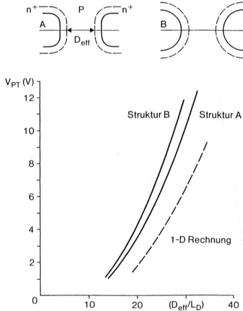
*Fig. 3:* Punch through voltage as a function of the normalized trench to trench distance for different trench geometries, as indicated in the insert.
