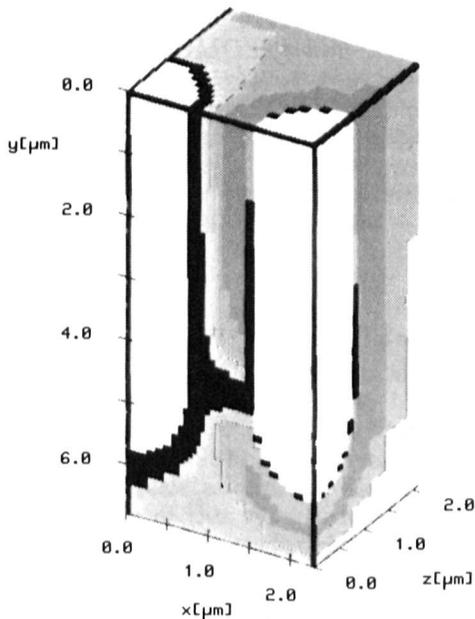
Fig. 7: Electron density distribution between two neighbouring trench capacitors for  $V_{tt} = 6 \text{ V}$ , the well type II and the geometry parameters  $T_1 = 5.5 \mu\text{m}$ ,  $R_1 = 0.55 \mu\text{m}$ ,  $R_2 = 0.4 \mu\text{m}$  and trench to trench distance  $D = 1.2 \mu\text{m}$ .
