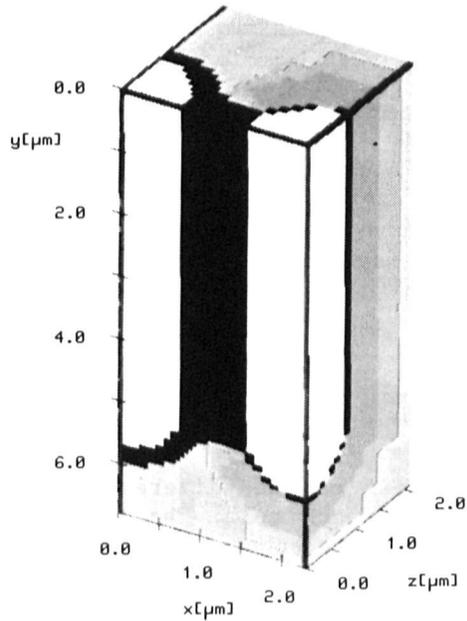
*Fig. 4:* Electron density distribution at  $V_{tt} = 6 \text{ V}$  for homogeneously doped substrate ( $2\text{E}16\text{cm}^{-3}$ ).
