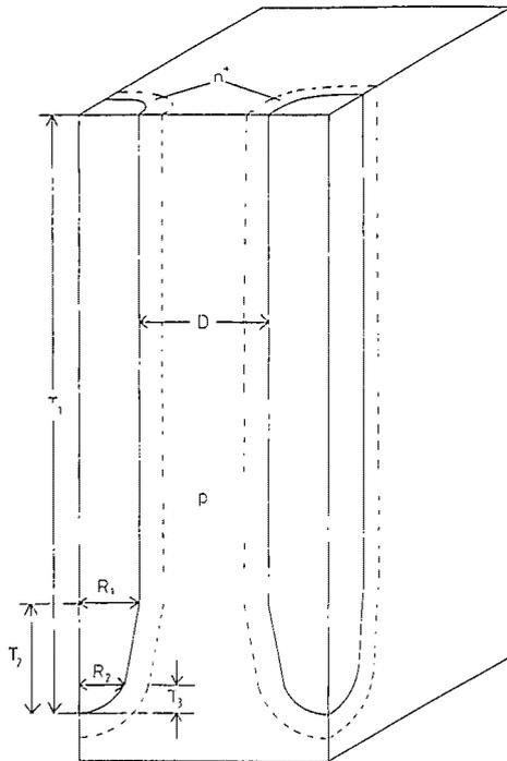
*Fig. 1:* Geometry of the simulated trench capacitor cell. The parameters are to be defined in the input file.
