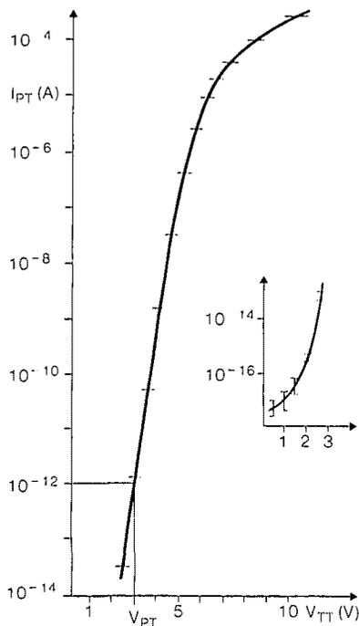
*Fig. 2:* Trench to trench leakage current as a function of the applied voltage.
