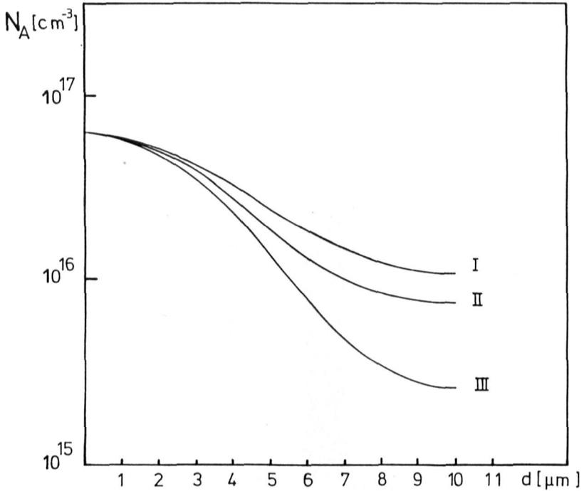
*Fig. 5:* Doping profile of the different p-wells used in the optimization of the trench cell. The concentration at large depths is identical to the substrate doping.
