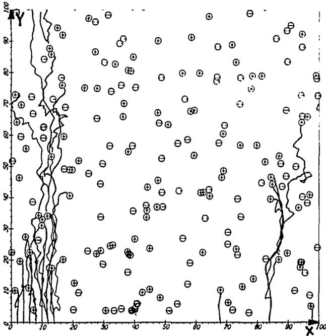
Fig. 6 Electrons trajectories calculated with the introduction of the electron-phonon scattering. Distribution of the centres is uncorrelated
