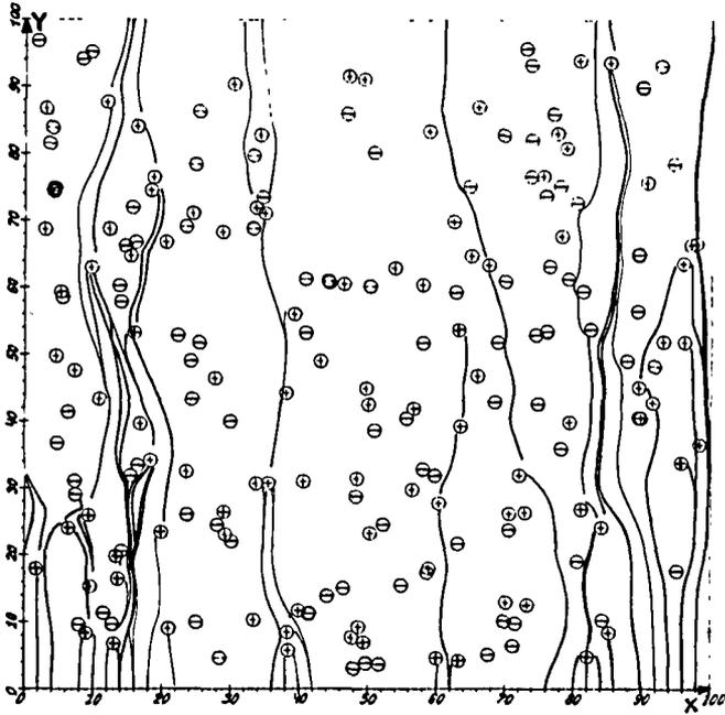
Fig. 5 Electrons trajectories. Distribution of the donors and acceptors is correlated.
