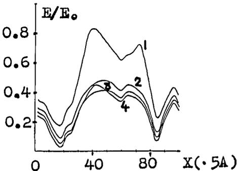
Fig. 4b Electric field strength at the boundary  $\text{SiO}_2\text{-Si}_3\text{N}_4$  for different time moments: 1- $t=0$ , 2- $t=10^{-3}$  s, 3- $t=10^{-5}$  s, 4- $t=10^{-8}$  s;  $E_0 = 8 \cdot 10^6$  v/sm, the rest parameters are the same Fig. 4a.
