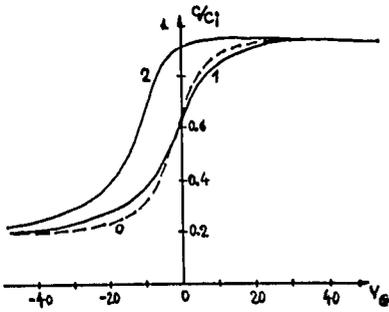
Fig. 4a C-V characteristics: "0"-ideal structure, "1"-initial, "2"- at the time  $t=10^{-3}$  s.  $C_i$  is the insulator capacity. Distribution of the centers is uncorrelated.  $V_G = 25 \text{ v}$ .
