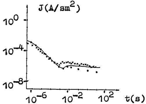
Fig. 7b Current through the structure vs time.  $T=300$  K, the rest parameters are the same as in Fig. 7a. ●●●● - experimental data [8], — - simulation results for diffusion-drift model [8], × - our calculation.
