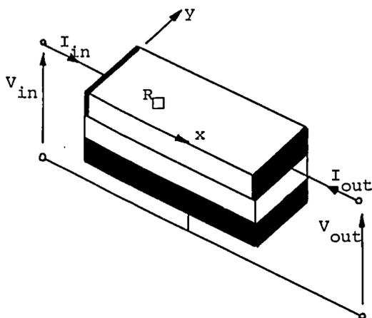
*Fig.1: Isometric view of the model for a polysilicon interconnect. The conducting top layer has a capacitance  $C$  per unit area with respect to the bottom layer.*
