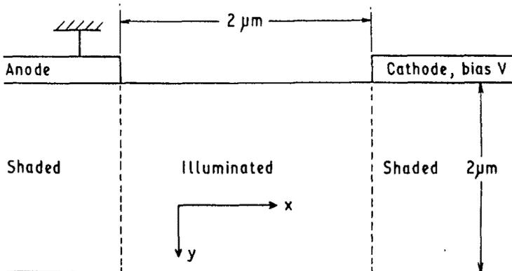
Fig 1: The GaAs photodetector geometry. The anode is earthed, the cathode biased. The coordinate system referred to in Eq. 9 is indicated here
