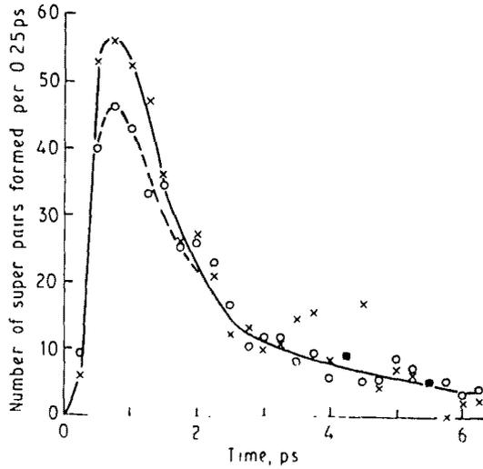
Fig 6: Number of electron-hole pairs created in intervals of 25 ps vs time for 3V bias (X) and the same bias with four times as many superparticles (--o--)
