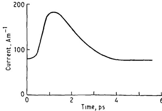
Fig 3: Cathode current vs time. It is obtained from the slope of the curve of Fig 2. The flash is applied at time 0.
