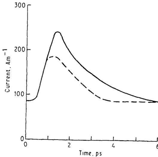
Fig 7: Cathode current vs time with and impact ionisation carrier multiplication (---) and with (---)
