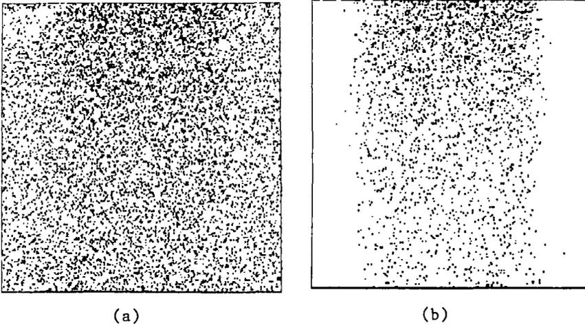
Fig 5: Momentary positions of (a) electrons and (b) holes in the photodetector
