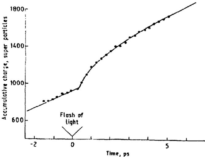
Fig 2: Accumulative super particles count at the cathode vs time. Each super particle represents a charge given by Eq.(7). The flash is applied at time 0.
