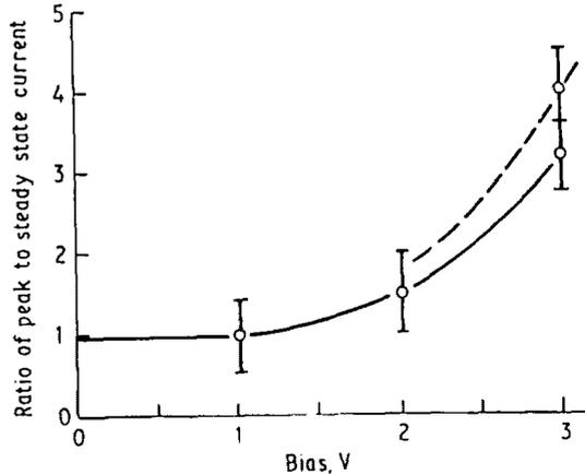
Fig 4: Ratio of peak and dark current vs applied bias.
