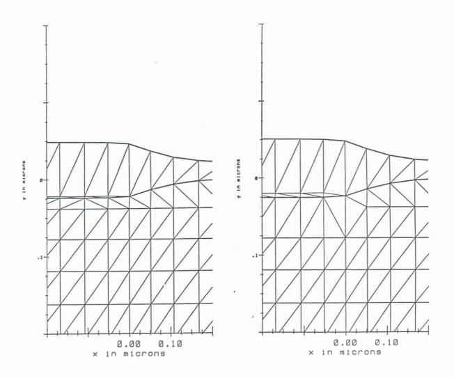
Figure 1. Silicon grid removal during oxidation
