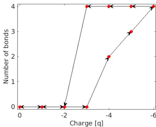
Fig.2: Number of interlayer bonds formed between a defective h-BN layer and its neighbors as a function of its charge. Increasing or decreasing the charge and minimizing the forces may result in a configuration change. Each arrow represents a different step, including a minimization of the force acting on the h-BN structure.
