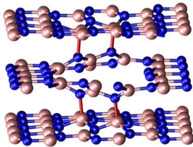
Fig.1: Representation of the atomic configuration of a triangular defect in h-BN where two bonds are formed between the defect and each adjacent layers. The blue and brown spheres represent N and B, respectively, and the interlayer bonds are marked in red.
