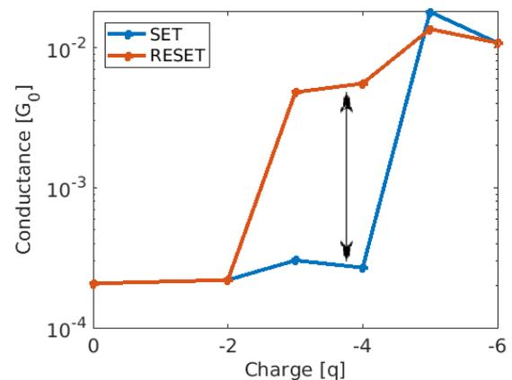
Fig.5: Conductance of the Au/h-BN/Au structure in Fig. 4 as a function of the charge during the SET and RESET processes. States with three or four interlayer bonds are conductive. Hence a hysteresis forms with an ON-OFF conductance ratio of more than one order of magnitude, as indicated by the black double arrow.
