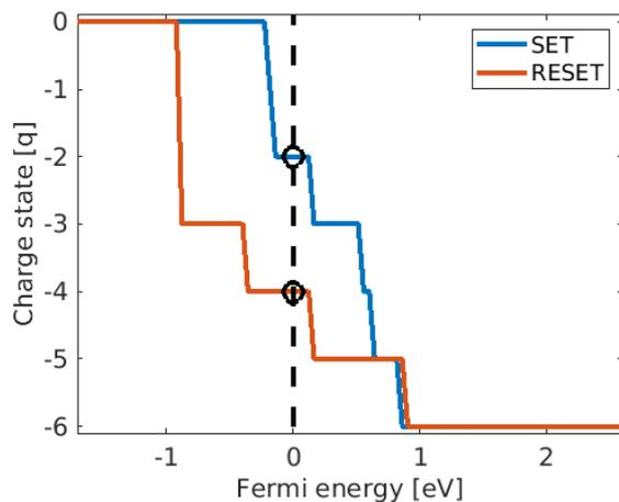
Fig.3: The preferred charge state of the triangular defect as a function of the Fermi energy. The SET and RESET potentials are around 1 eV and -1 eV. These are probably underestimated due to the nature of the PBE functional employed in DFT. The dashed black line indicates the equilibrium potential when the h-BN is in contact with Au. The upper (lower) black circle mark the equilibrium OFF- (ON-) state.
