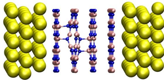
Fig.4: Schematic view of the Au/h-BN/Au structure used to evaluate defect-induced conductance changes. The yellow spheres represent the Au contact atoms. The entire structure is optimized with DFT.
