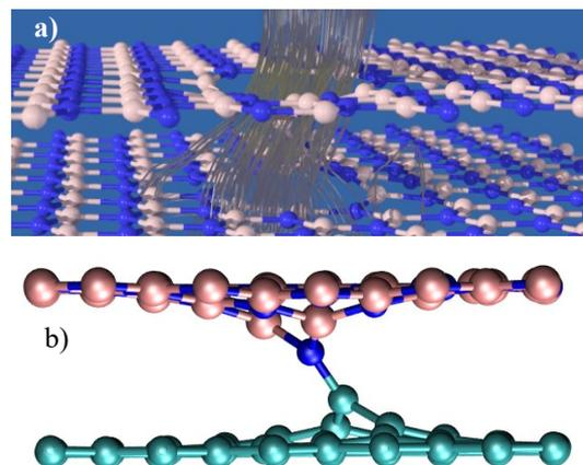
Fig.6: a) The gray lines are an illustration of the current flowing through a defect in h-BN with a single interlayer bond. The pink and blue spheres are the B and N atoms, respectively. b) Example of a defect forming a bond between an h-BN layer and a graphene electrode, where the cyan spheres represent C atoms. The resulting bonding could induce a similar resistance switching characteristic as the one presented here for bulk h-BN.
