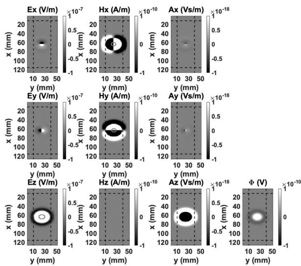
Fig.1: Snapshot of fields and potentials for FiPo FDTD at 0.32 ns.
