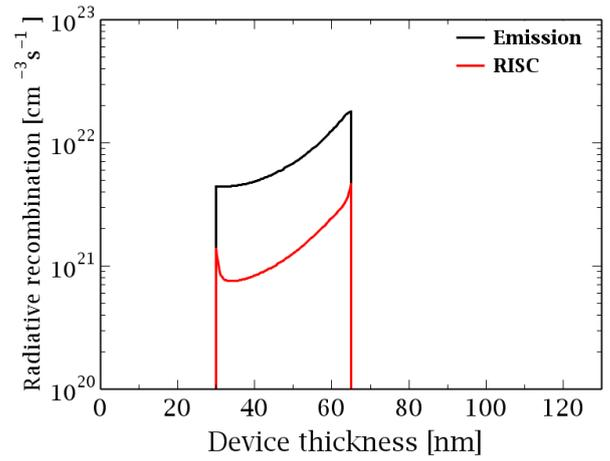
Fig.3: Radiative emission profile (black) and reverse inter-system crossing rate (red) calculated with mp-DD simulation at 6V bias operation within the emitter of a TADF OLED consisting of a TCTA/CBP:4CzIPN/TBPi stack.
