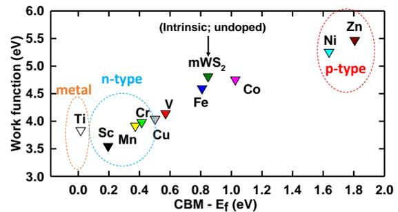
Fig.6: The work function versus the energy difference between the conduction band minimum (CBM) and the fermi level ( $E_f$ ) of the TM-doped mWS<sub>2</sub>.
