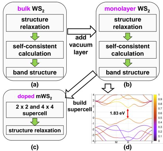
Fig.2: The simulation flow from (a) bulk WS<sub>2</sub> to (c) doped monolayer WS<sub>2</sub>. (d) The obtained monolayer WS<sub>2</sub> band structure. The color bars indicate the weighting of band dominated by tungsten atoms. The direct bandgap is 1.83 eV for monolayer WS<sub>2</sub>.
