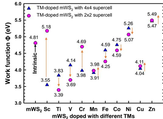
Fig.5: The work function of TM-doped mWS<sub>2</sub> with respect to different TM materials. The triangle and circle symbols are results of  $4 \times 4$  and  $2 \times 2$  supercells, respectively. The most stable structure, I-T, is simulated with two different doping concentrations. The arrows indicate how the work function changes as the doping concentration increases.
