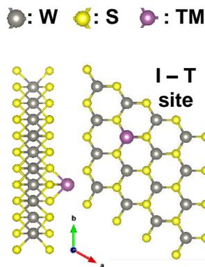
Fig.4: The most stable doped structure of mWS<sub>2</sub> of four possible doping sites is I-T site, the gray, yellow, and brown atoms are W, S, and doping transition metal, respectively. Two interstitial (I) and two substitutional (S-) sites are simulated to determine the most stable site with lowest formation energy.
