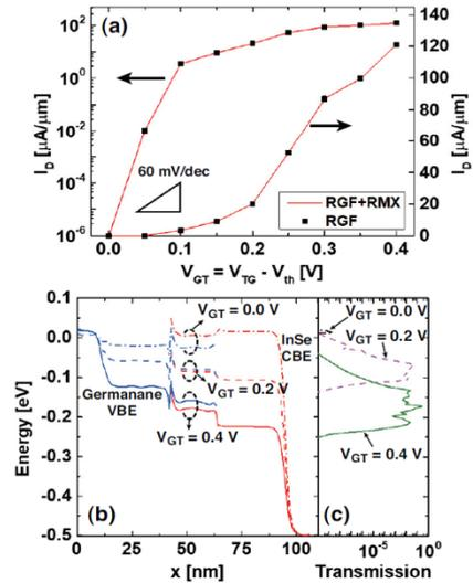
Fig.5 (a) Transfer characteristics of the simulated germanane/InSe vertical TFET at drain voltage of 0.4 V and top gate voltage ( $V_{TG}$ ) of -0.8 V. Threshold voltage ( $V_{th}$ ) is defined such that off-state current is  $10^{-6} \mu A/\mu m$ . (b) Band edge profile and (c) transmission (log scale) of the simulated vertical TFET at various top gate voltages.  $V_{GT}$  denotes  $V_{TG}-V_{th}$ .
