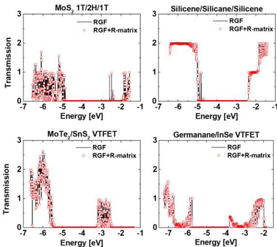
Fig.3: The transmission functions of the simulated heterostructures.
