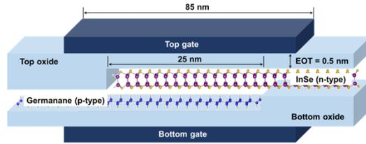
Fig.4: Schematic of the simulated germanane/InSe vertical TFET.
