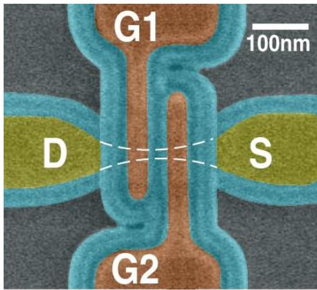
Fig.1: SEM image of a SOI device. The gates G1 and G2 control two quantum dots along a  $[110]$  Si nanowire outlined by the dashed white lines. The dot under G1 is used as a filter to measure the spin in the qubit under G2 through Pauli spin blockade of the source-drain (SD) current. The qubit is manipulated by radio-frequency pulses on G2 [1].
