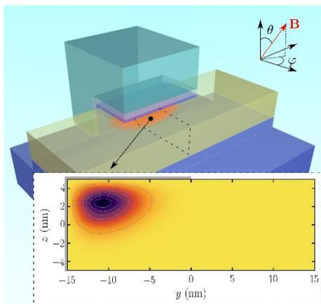
Fig. 3: 3D model of a SOI device with a Si nanowire in yellow, SiO<sub>2</sub> in dark blue, and a partly overlapping gate in light blue. The location of the electron trapped under the gate is sketched in orange. A map of the squared wave function is plotted in the cross-section outlined by the dashed black lines. The orientation of the magnetic field  $\mathbf{B}$  (see Fig. 5) is characterized by the angles  $\theta$  and  $\phi$ .
