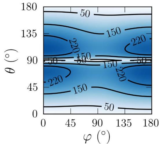
Fig. 5: Map of the Rabi frequency (MHz) of a heavy-hole spin qubit as a function of the orientation of the magnetic field, characterized by the angles  $\theta$  and  $\phi$  (see definition on Fig. 3) [4].
