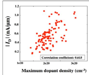
Fig. 6. Scatter plot of drain currents and maximum dopant density.
