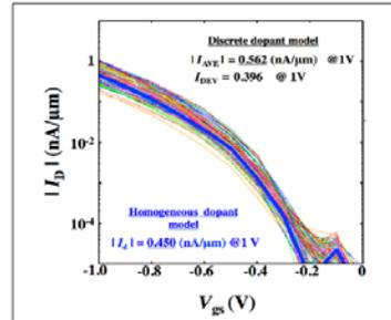
Fig. 2.  $I_D - V_{GS}$  curves for 100 TFETs with discrete dopant distributions.
