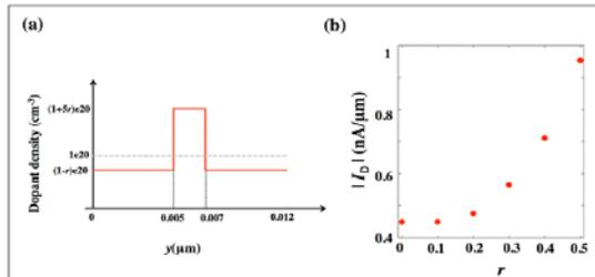
Fig. 4. (a) Non-uniform dopant density distribution with localization strength  $r$ , and (b) drain current  $I_D$  as a function of  $r$ .
