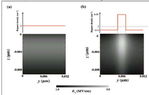
Fig. 5. (a) Distributions of  $E_x$  at the source edge region ( $x = 0.057 \mu\text{m}$ ) of (a) uniform model and (b) non-uniform model.
