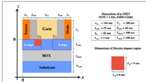
Fig. 1. Schematic figure of TFET with discrete dopant distribution (shaded area).
