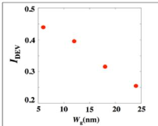
Fig. 3. Relative standard deviations of drain currents  $I_{DEV}$  as a function of device width  $W_g$ .
