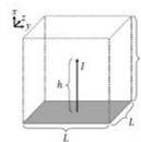
Fig. 3. Monopole radiation is simulated by using AC NEGF to simulate transport in a 1D metal wire with length  $h = 770 \mu\text{m}$  in an FDFD simulation of side length  $L = 1.73 \text{ mm}$ . Perfect electrical conductor electromagnetic boundary conditions are applied on  $y = z$  plane, shown as the solid gray cube face, while absorbing boundary conditions are applied to all other faces, illustrated as transparent faces with dashed edges.
