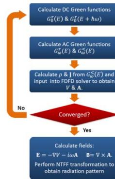
Fig. 2. Solution procedure to achieve self-consistent electrodynamic fields with AC NEGF.
