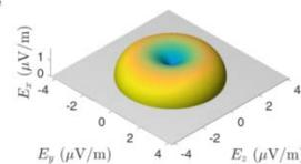
Fig. 4. The far-field radiation pattern at a distance  $r = 1 \text{ cm}$  obtained by performing a near-to-far-field transformation of the electric and magnetic fields outside the wire. We see that the antenna radiates as a quarter-wave monopole thereby demonstrating the ability of this method to capture radiative electrodynamic phenomena.
