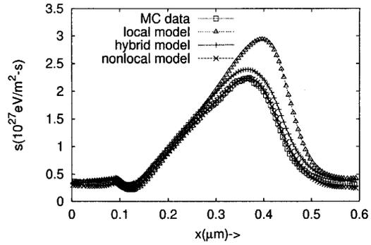
Fig. 8 Comparison of  $s$  predicted by the local model, the hybrid model and the non-local model with that of MC data.
