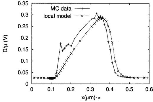
Fig. 6 Comparison of  $D/\mu$  predicted by the local energy-dependent model with that of actual MC simulation data.
