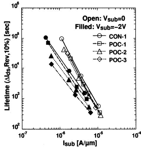
Figure 6: Measured device lifetime as a function of  $I_{sub}$ . The lifetime is evaluated by 10 % degradation of S/D-reversed  $I_{ds}$ . The stress bias condition for  $V_g$  is chosen to give  $I_{sub, max}$  at each  $V_d$  in  $V_{sub} = 0, -2$  V cases.
