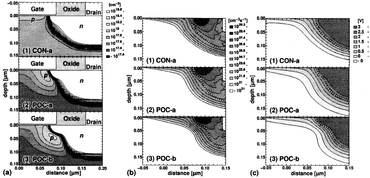
Figure 1: (a) Device structure for simulation, (b) calculated electron impact ionization generation rate, and (c) calculated potential distribution of three 0.18  $\mu\text{m}$  nMOSFETs at  $V_g = 1.7$  V,  $V_d = 3$  V. The origin is at gate center and silicon/gate-oxide boundary. Dotted lines denote  $pn$ -junction.
