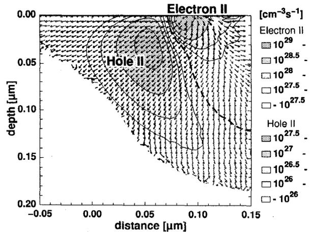
Figure 3: Distribution of electron and hole impact ionization generation rates (contour) and hole current (allows) of POC-a at  $V_g = 1.7 \text{ V}$ ,  $V_d = 3 \text{ V}$ . Dashed line denotes the pn-junction.
