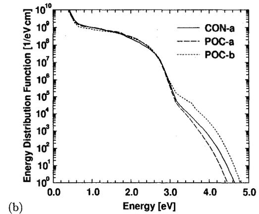
Figure 2: (a) Flux of electrons which hit the silicon/gate-oxide boundary and (b) energy distribution function of electrons in the whole silicon region at  $V_g = 1.7 \text{ V}$ ,  $V_d = 3 \text{ V}$ .
