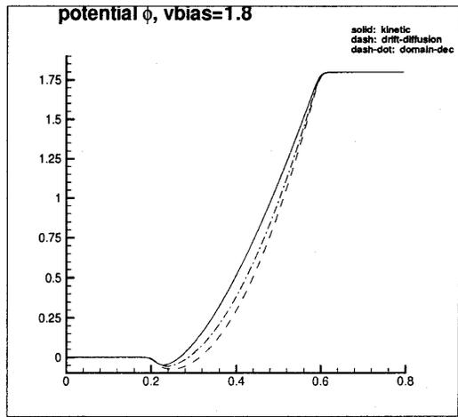
Figure 7: The potential  $\phi$ .  $\mu = \mu(E)$ .  $vbias = 1.8V$ . Comparison among the kinetic result (solid line), the low field drift-diffusion among the kinetic result (solid line), the low field drift-diffusion model (dashed line), and the elementary domain decomposition with low field drift-diffusion in  $[0,0.25]$  and  $[0.55,0.8]$ , and high field model in  $(0.25,0.55)$  (dash-dotted line).
