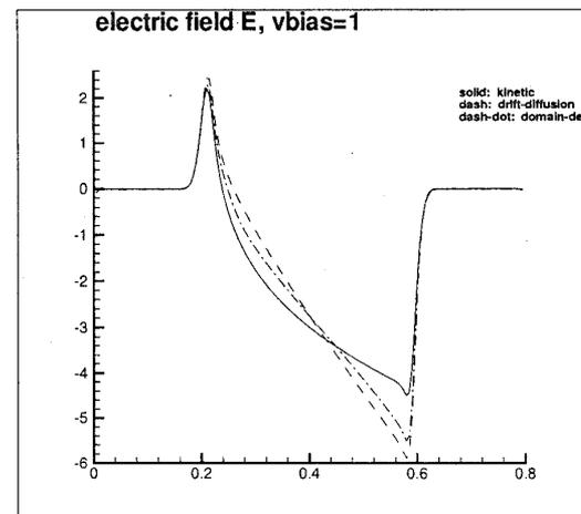
Figure 3: The electric field  $E$ .  $\mu = \mu(E)$ .  $v_{bias} = 1V$ . Comparison among the kinetic result (solid line), the low field drift-diffusion model (dashed line), and the elementary domain decomposition with low field drift-diffusion in  $[0,0.27]$  and  $[0.55,0.8]$ , and high field model in  $(0.27,0.55)$  (dash-dotted line).
