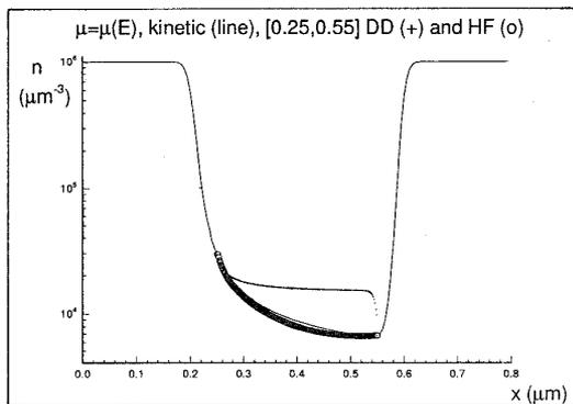
Figure 1: The global kinetic simulation (solid line), the mid-region HF simulation (circles), and the mid-region DD simulation (plus signs).  $\mu = \mu(E)$  for all simulations. The global kinetic simulation provides the boundary conditions for the mid-region HF and DD simulations. The concentration  $n$  in  $\mu m^{-3}$ .
