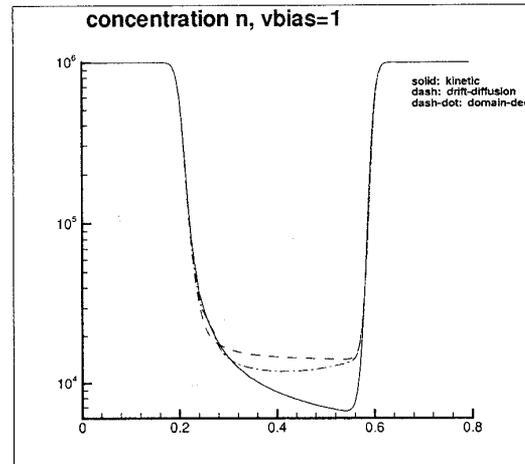
Figure 2: The concentration  $n$ .  $\mu = \mu(E)$ .  $v_{bias} = 1V$ . Comparison among the kinetic result (solid line), the low field drift-diffusion model (dashed line), and the elementary domain decomposition with low field drift-diffusion in  $[0,0.27]$  and  $[0.55,0.8]$ , and high field model in  $(0.27,0.55)$  (dash-dotted line).
