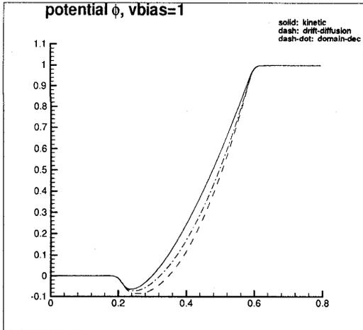
Figure 4: The potential  $\phi$ .  $\mu = \mu(E)$ .  $vbias = 1V$ . Comparison among the kinetic result (solid line), the low field drift-diffusion model (dashed line), and the elementary domain decomposition with low field drift-diffusion in  $[0,0.27]$  and  $[0.55,0.8]$ , and high field model in  $(0.27,0.55)$  (dash-dotted line).
