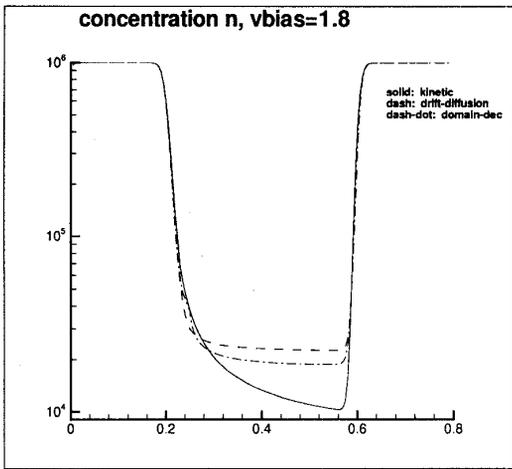
Figure 5: The concentration  $n$ .  $\mu = \mu(E)$ .  $vbias = 1.8V$ . Comparison among the kinetic result (solid line), the low field drift-diffusion model (dashed line), and the elementary domain decomposition with low field drift-diffusion in  $[0,0.25]$  and  $[0.55,0.8]$ , and high field model in  $(0.25,0.55)$  (dash-dotted line).
