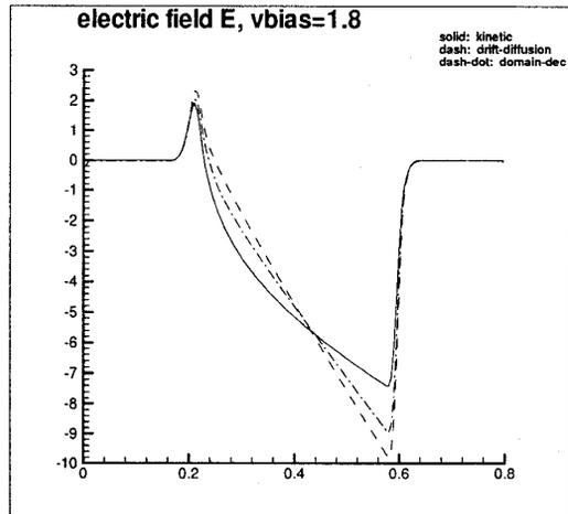
Figure 6: The electric field  $E$ .  $\mu = \mu(E)$ .  $vbias = 1.8V$ . Comparison among the kinetic result (solid line), the low field drift-diffusion among the kinetic result (solid line), the low field drift-diffusion model (dashed line), and the elementary domain decomposition with low field drift-diffusion in  $[0,0.25]$  and  $[0.55,0.8]$ , and high field model in  $(0.25,0.55)$  (dash-dotted line).
