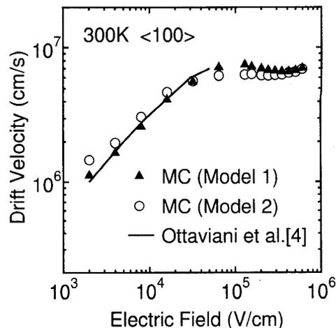
Figure 2: Experimental and simulated hole drift velocity at room temperature as a function of electric field along the (100) crystallographic direction.
