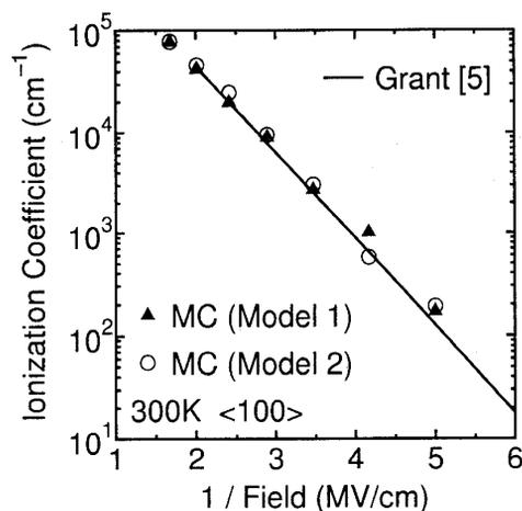
Figure 3: Experimental and simulated impact ionization coefficient at room temperature for a field along the (100) crystallographic direction.
