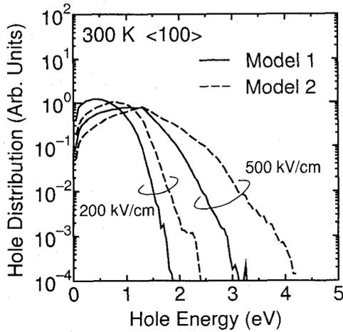
Figure 4: Calculated hole energy distributions at room temperature in the homogeneous electric fields along the  $\langle 100 \rangle$  crystallographic direction.
