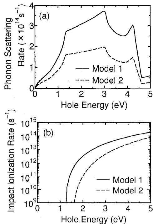
Figure 1: Hole energy dependence of the scattering rates compared in this study. (a) Hole-phonon and (b) hole initiated impact ionization scattering rates.
