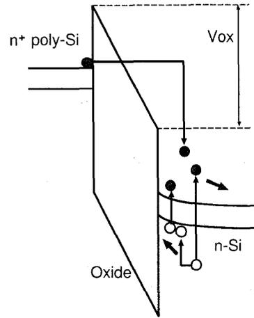
Figure 6: Schematic energy band diagram illustrating quantum yield experiment. This figure shows two impact-ionization events initiated by an electron injected from  $\text{SiO}_2$  and a secondary generated hole.
