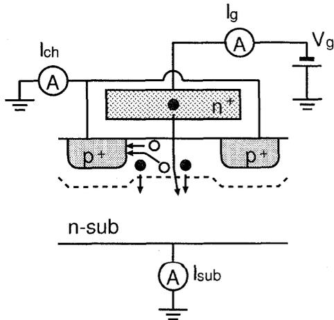
Figure 5: Schematic picture of the experimental setup of charge separation technique to measure the quantum yield of impact ionization. Closed and open circles represent electrons and holes, respectively.
