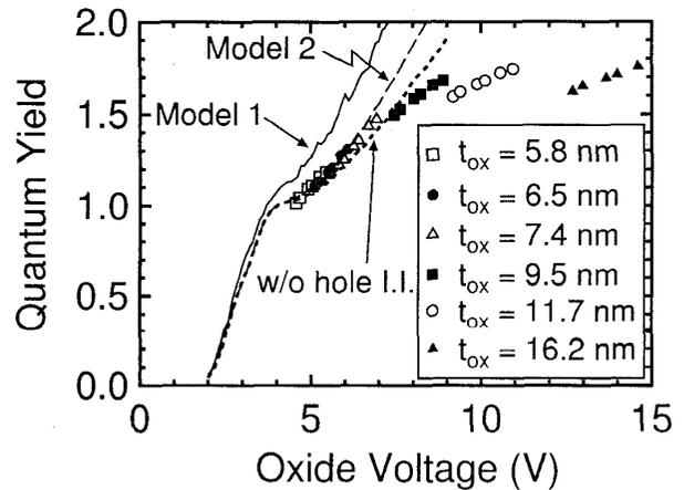
Figure 7: Experimental (symbols) and calculated (lines) data of quantum yield as a function of oxide voltage.
