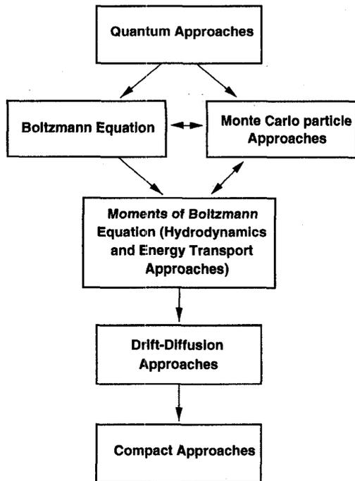
Figure 1: Schematic diagram illustrating the simulation hierarchy
