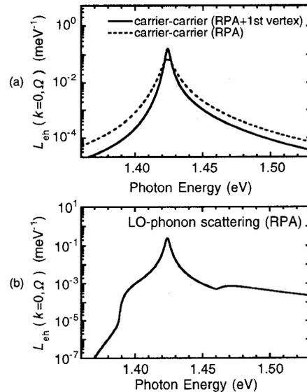
Figure 1: Photon spectral shape functions at band edge ( $k=0$ ) with (a) carrier-carrier scattering and (b) carrier-LO phonon scattering.
