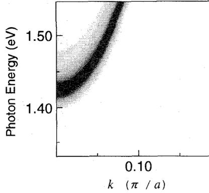
Figure 3: Energy-momentum diagram of photon spectral shape function.
