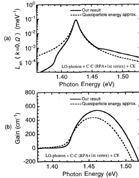
Figure 5: Comparison between our result and quasiparticle energy approximation for (a) photon spectral shape functions at  $k=0$  and (b) optical gain spectra.
