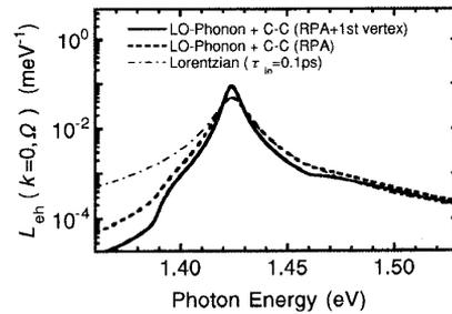
Figure 2: Total photon spectral shape function at  $k=0$ .
