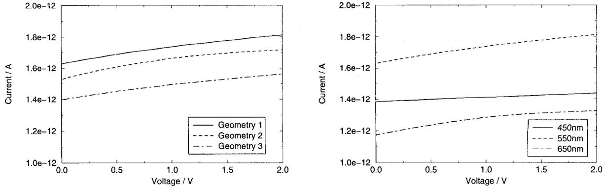
Figure 2: Quasistationary current due to photo-generated carriers at the CCD's photodiode for different geometries at  $\lambda = 550\text{nm}$  (left) and for Geometry 1 at different illumination wavelengths (right) as a function of the (reverse bias) voltage  $U$  applied to the  $n^-$  doping region..
