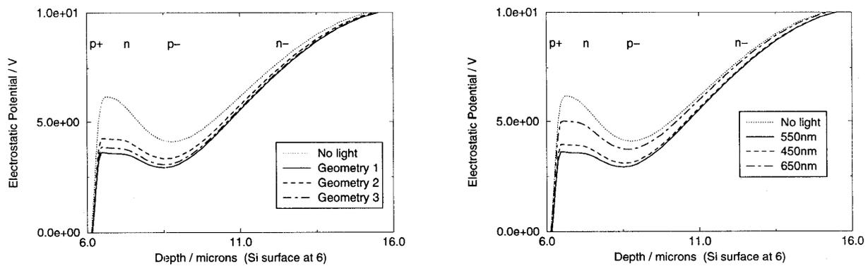
Figure 3: Transient electrostatic potential reduction due to photo-generated carriers in the CCD geometries at  $\lambda = 550\text{nm}$  (left) and for Geometry 1 at different illumination wavelengths (right).
